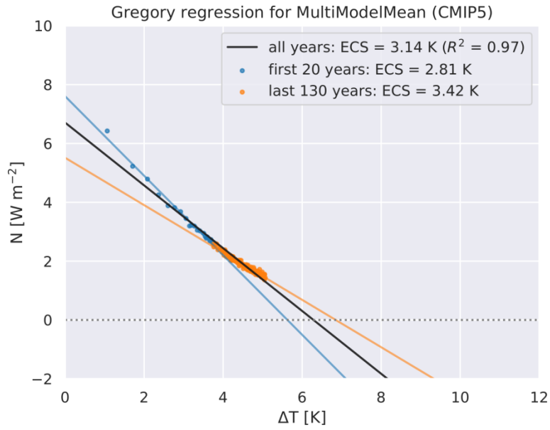
850 Figure 3 Gregory plot to approximate the effective climate sensitivity (ECS) (Gregory et al., 2004). Shown is the relationship between the differences in global and annual mean top of the atmosphere net downward radiative flux N ( \text{W m}^{-2} ) and global and annual mean near-surface air temperature anomalies \Delta T (K) for the CMIP5 multi-model mean. Anomalies are calculated as difference between the abrupt4xCO 2 experiment (quadrupling of CO 2 ) and the pre-industrial control run (piControl). The blue dots show the first 20 years of the simulation, the orange dots the last 130 years. A linear regression using only the first 855 20 years (blue line) instead of all 150 years (black line) results in a stronger feedback (and thus lower ECS). Using the last 130 years only (orange line) results in a weaker feedback (i.e. higher ECS). See Section 3.2 for details on recipe_ecs.yml .
