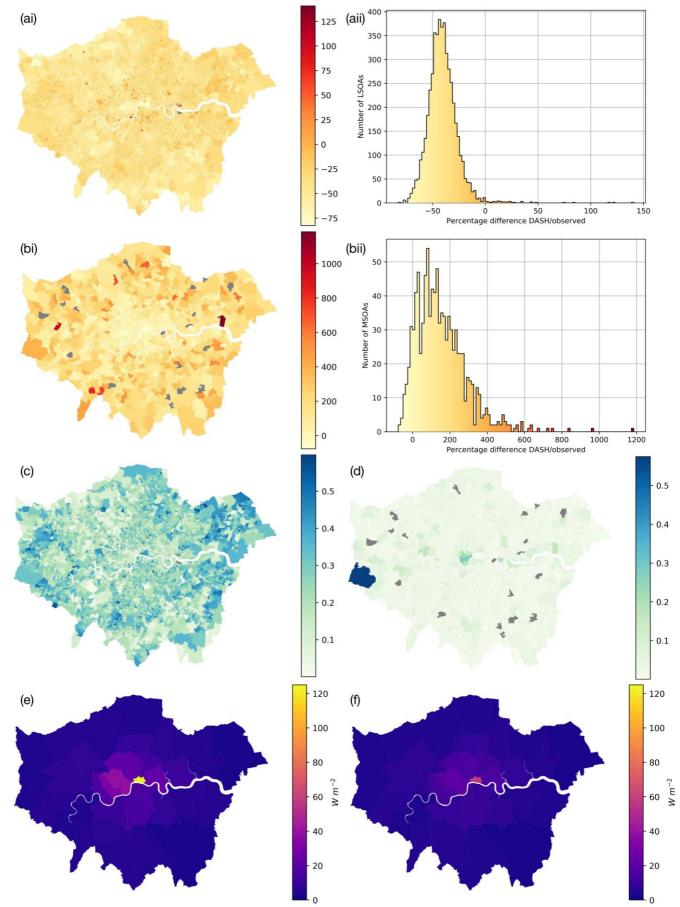
Figure 11: DASH (R8, Table 6)  $nE_i$  of total energy consumption represented by (i) choropleth and (ii) histogram for (a) LSOA scale domestic use and (b) MSOA scale commercial use. AnE<sub>i</sub> of total energy consumption for (c) LSOA scale domestic and (d) MSOA scale commercial. Annual average energy consumption at LA scale for (e) reference data and (f) DASH.
