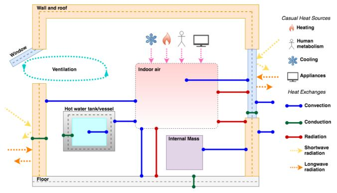
**Figure B1:** STEBBS 1-D model simulates building facets/nodes (dots), casual heat sources and heat exchanges. Longwave radiation is absorbed by building facets from the outdoor environment, and shortwave radiation from direct, diffuse and reflected sources.
