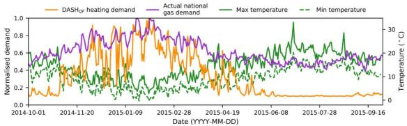
1165 Figure 10: Daily (1 October 2014 - 30 September 2015) DASH normalised total heating/cooling and domestic hot water (DHW) energy demand (R7, Table 6) for Greater London, minimum and maximum London outdoor air temperature (°C) (Table 5) and normalised national gas demand (NG, 2015). See section 3.2 for normalisation.
