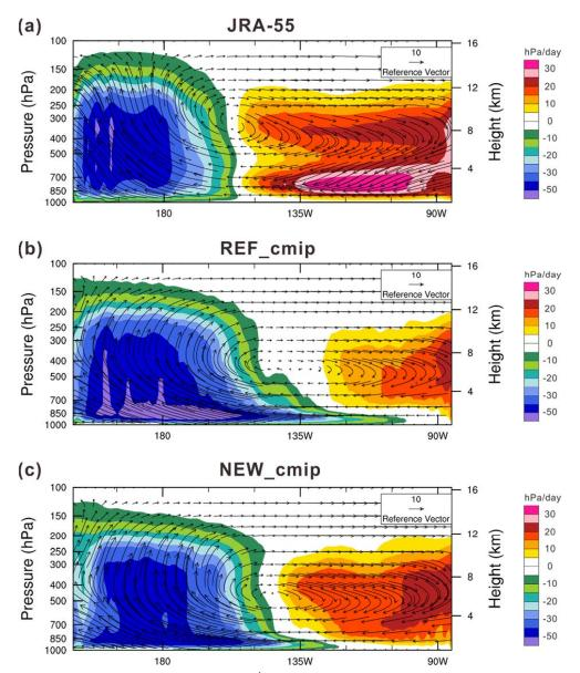
Figure 9. Annual mean vertical pressure velocity (hPa day  $^{-1}$ ; shaded) and wind vectors (arrows) in the longitude-height cross section averaged over  $5^{\circ}S - 10^{\circ}S$  for (a) the JRA-55 reanalysis, (b) REF\_cmip, and (c) NEW\_cmip.
