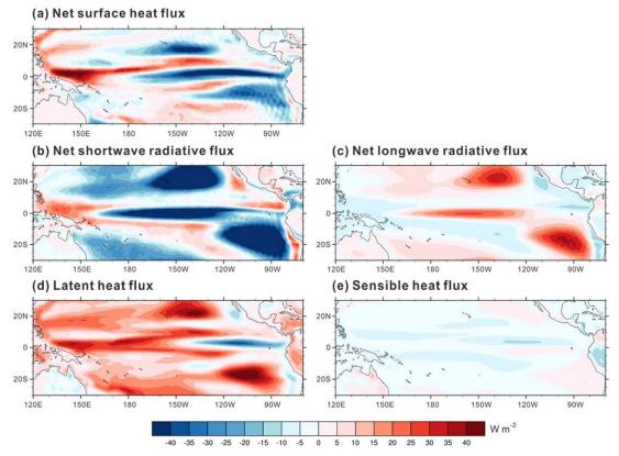
Figure 8. The differences between the NEW\_cmip and REF\_cmip simulations (W m<sup>2</sup>) for (a) net surface heat flux  $\Delta Q_{alm}$ , (b) net shortwave radiative flux  $\Delta Q_{SW}$ , (c) net longwave radiative flux  $\Delta Q_{LW}$ , (d) latent heat flux  $\Delta Q_{LH}$ , and (e) sensible heat flux  $\Delta Q_{SH}$ .
