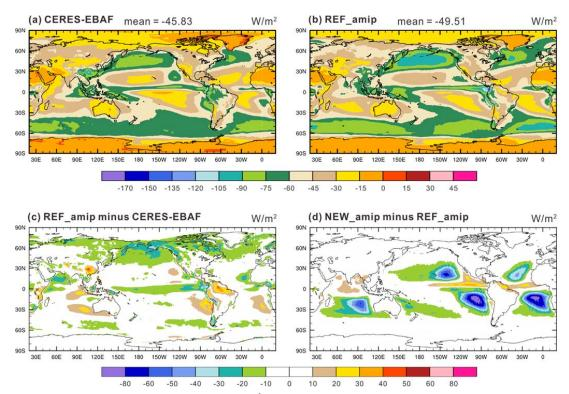
Figure 1. Annual mean climatologies of TOA SWCRF (W m<sup>-2</sup>) from (a) CERES-EBAF observations (from 2001 to 2010), (b) REF\_amip, and the differences between (c) REF\_amip and observations, (d) NEW\_amip and REF\_amip. Shown atop panels (a) and (b) are global mean values.
