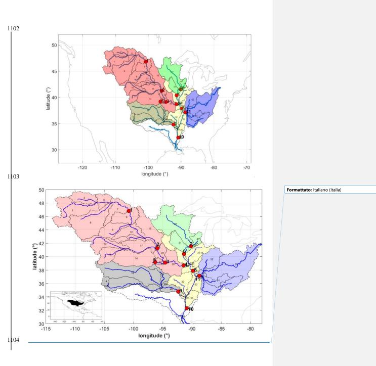
Figure 3. Mississippi sub-basin delineation. Red dots indicate the location of the discharge gauging stations; different colours identify different inner sections (and the related contributing sub-basins) used for the model calibration.
