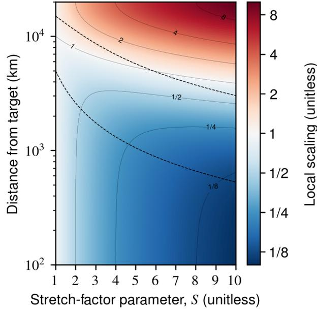
**Figure 3.** Local scaling as a function of distance from the target point, for stretch-factors in the range 1–10. The dashed lines show the distance from the target point to the cubed-sphere face edges after stretching. The lower dashed line is the distance to the center of the target-face’s edges, and the upper dashed line is the distance to the center of the opposite face edges.
