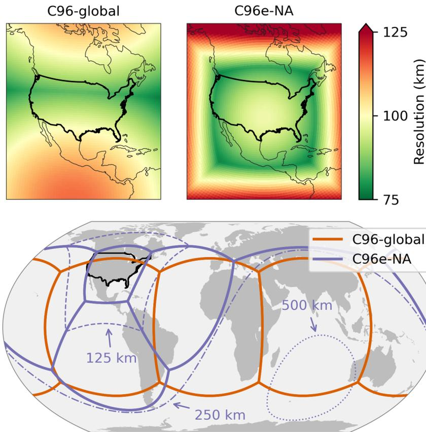
**Figure 4.** Comparison of C96-global and C96e-NA grids. The top panels show the variability of resolution for both grids. The bottom panel shows the grid face edges for C96-global and C96e-NA, with the 125 km, 250 km, and 500 km resolution contours for C96e-NA.
