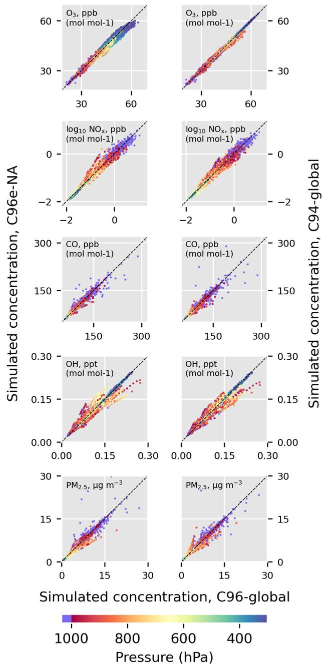
**Figure 5.** Comparison of simulated concentrations from C96e-NA with C96-global, and C94-global with C96-global. Points are 1-month time averages for each grid-box in the contiguous US for the fourth simulation month (September 2018). The right column gauges expected differences due to the precision of upscaling emissions to different grids. Concentrations in the lowermost model level are shown in purple.
