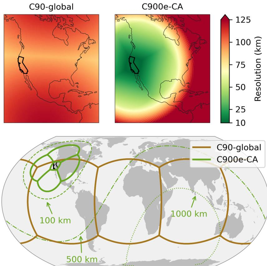
**Figure 8.** Comparison of C90-global and C900e-CA grids. The top panels show the variability of resolution for both grids. The bottom panel shows the grid face edges for C90-global and C900e-CA, with the 100 km, 500 km, and 1000 km resolution contours for C900e-CA.
