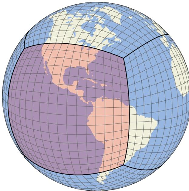
**Figure 1.** Illustration of a C16 grid. A cubed-sphere grid always has six faces. One of the six faces is highlighted for illustrative purposes. The highlighted face is a  $16 \times 16$  grid that is regularly spaced in a gnomonic projection centered on the face.
