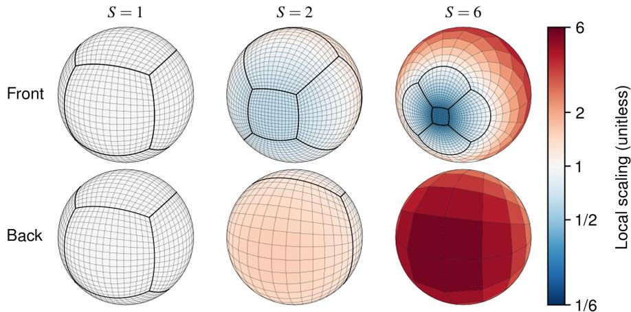
**Figure 2.** Three stretched-grids that illustrate the effect of the stretch-factor ( $S$ ) on stretching a C16 cubed-sphere. Local scaling is the relative change to a grid-box's edge length induced by stretching.
