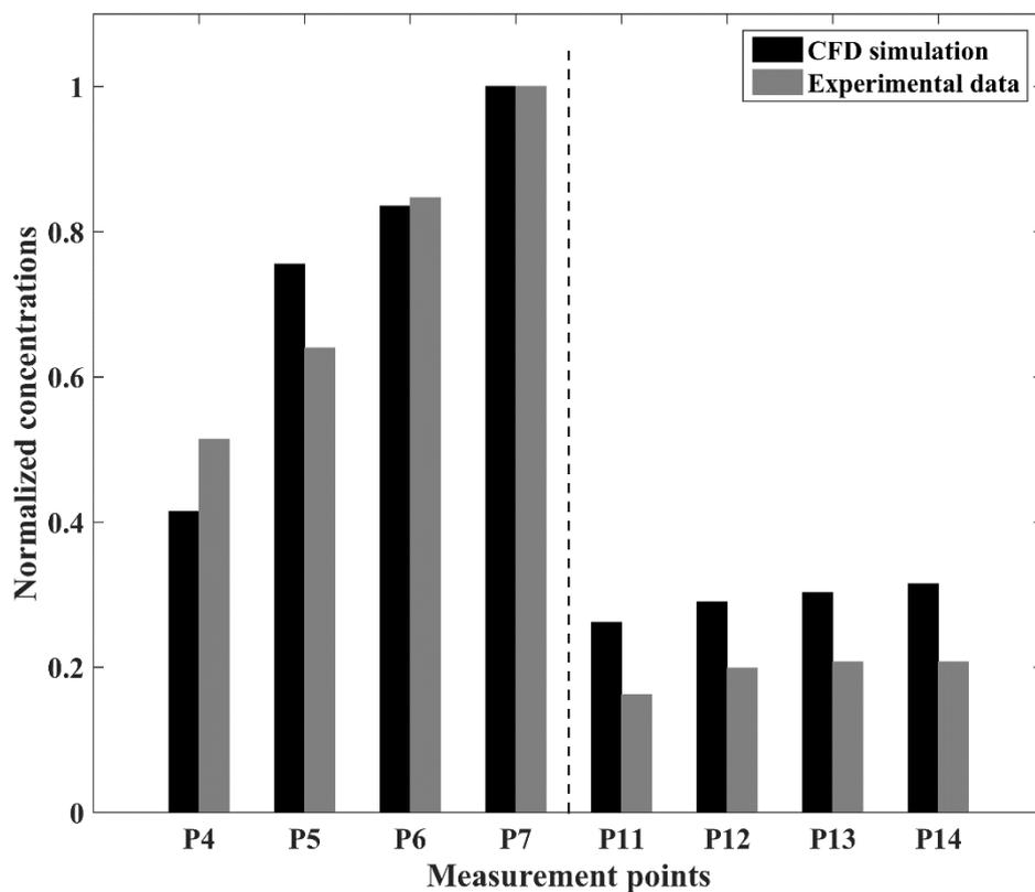
735 **Figure 8. Normalized concentrations of CFD and experimental data at each measurement point in 2D dispersion case**
