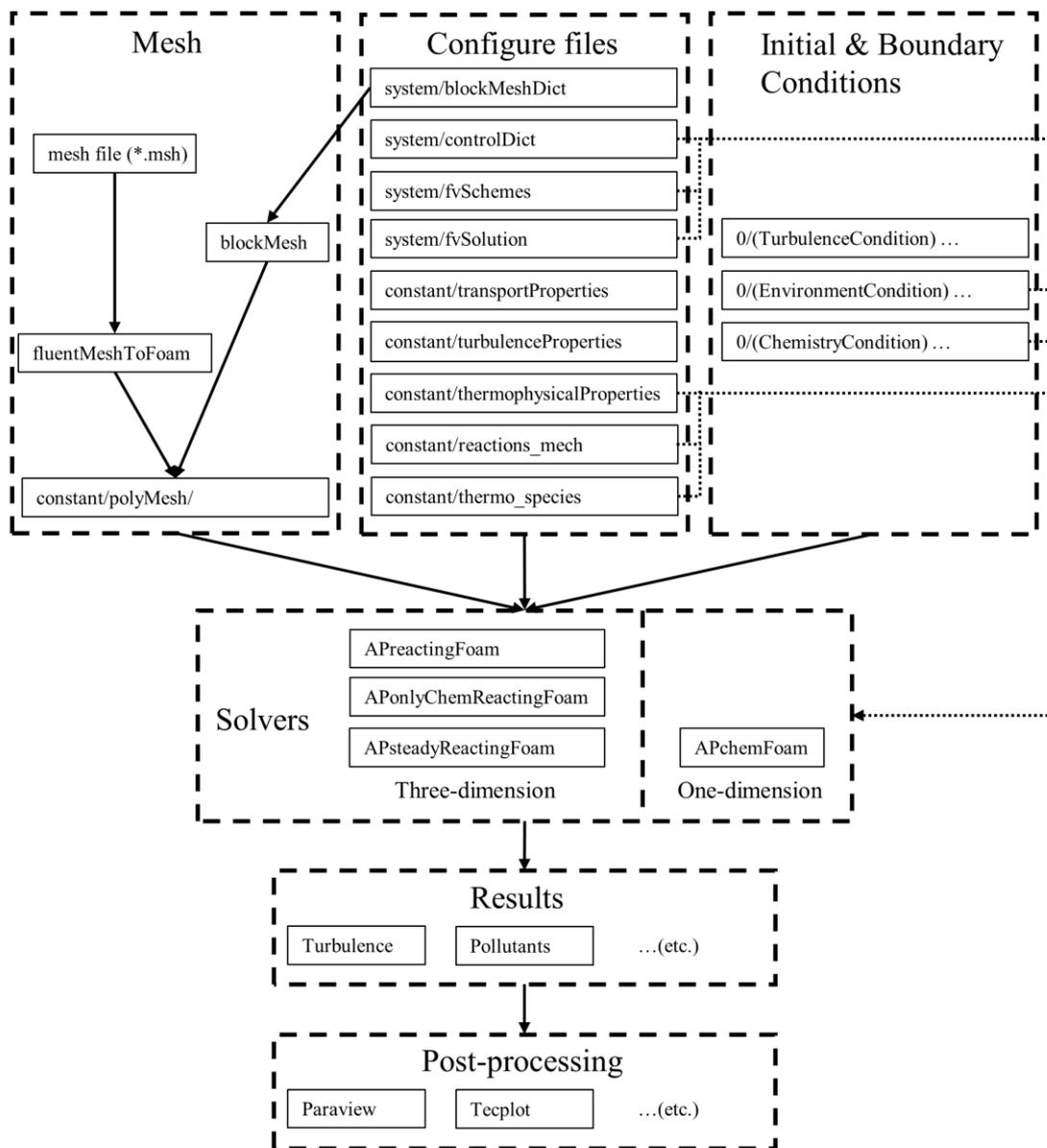
710 **Figure 1. Flow diagram of simulation set-up in APFoam framework**
