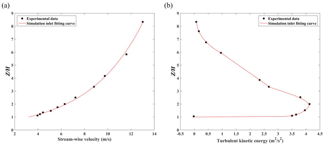
725 Figure 5. The inlet profile of (a) stream-wise velocity and (b) turbulent kinetic energy in single street canyon case
