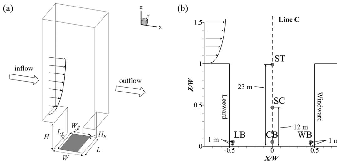
**Figure 9. Schematic diagram of (a) the CFD simulation domain and (b) the probe points location**
