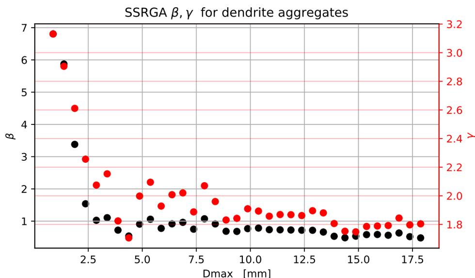
**Figure 1.** Example of the evolution of the fitted SSRGA parameters  $\beta$  (black) and  $\gamma$  (red) as a function of the snowflake maximum diameter for a aggregates of dendrites. Note that the scales for the two quantities are different and that they are reported at the opposite sides of the graph.
