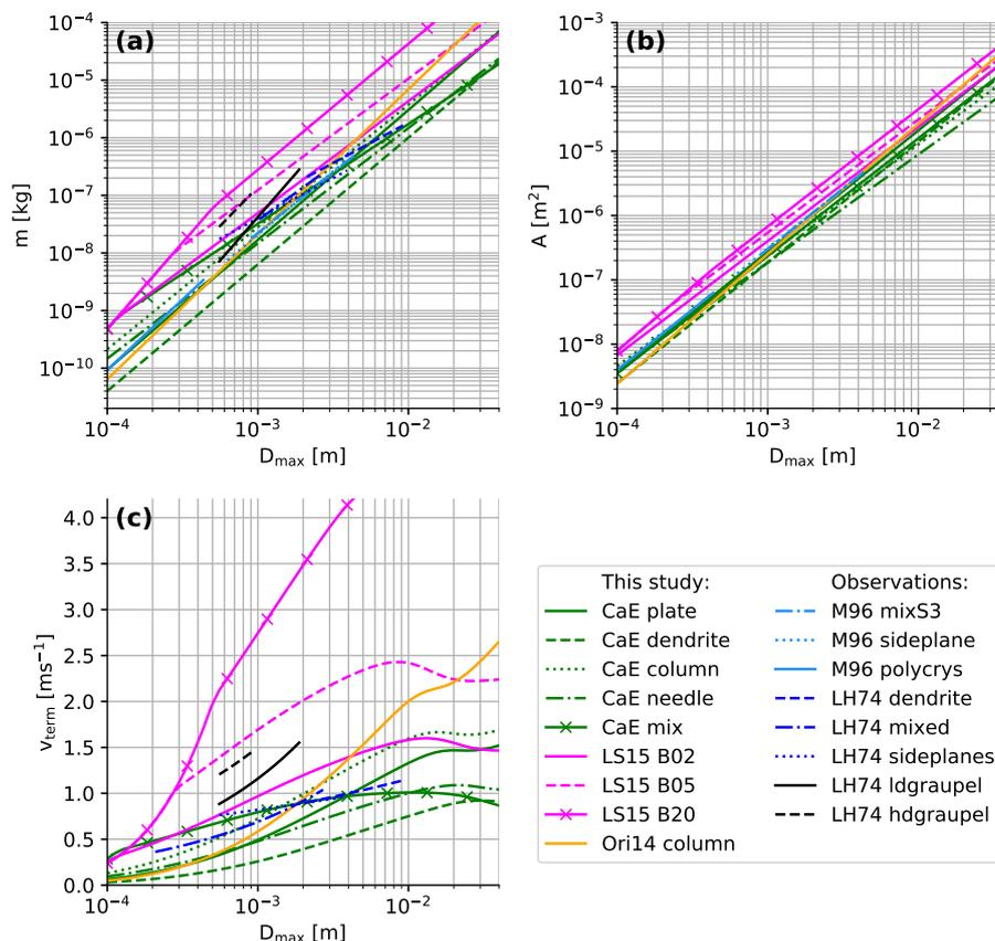
**Figure 4.** Mass a), projected area b) and terminal velocity c), of a selection of the simulated aggregates included in snowScatt and two frequently used in-situ studies (Locatelli and Hobbs, 1974; Mitchell, 1996). Terminal fall velocity in c) is calculated using the hydrodynamic model from Böhm (1992).
