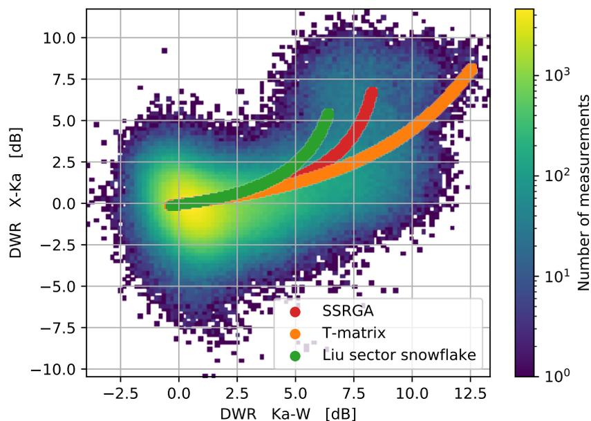
**Figure 9.** 2d-histogram of DWR X-Ka and Ka-W measured on during the TRIPEX campaign (Dias Neto et al., 2019) at the JOYCE supersite on 24 November 2015. The three colored curves show the simulated DWR-DWR relations based on the ICON-P3 model output and the three scattering methods used (SSRGA, T-matrix and DDA).
