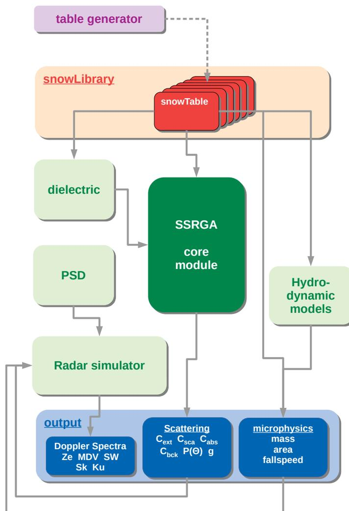
**Figure 2.** Schematics of the modules included in the snowScatt package and basic workflow. The various components are color-coded according to their primary use. The reddish and green blocks identify respectively the data and algorithmic components of the package. The auxiliary “table generator” package, that can be used to extend the snowLibrary database, is colored in violet. Even though the output is not technically a module of the snowScatt package it is here highlighted in blue coloring.
