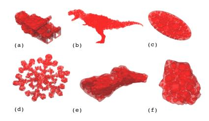
Figure 4. Application of the pre-processing routine *fromStlToSpheres* to objects characterized with different surfaces (i.e. convex hulls or not) that will be used in this paper. In (a) a LEGO toy, in (b) a T-rex, in (c) an ellipsoid, in (d) a snowflake, in (e) and (f) two different volcanic particles. No scale has been reported for this image since it is not important for the pre-processing. In fact, all the objects will be rescaled by the mainSCARLET function.
