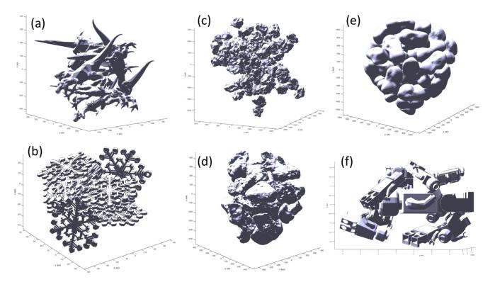
Figure A1. Virtual aggregates made of different initial stl files. (a) aggregate made from a stl file of a t-rex; (b) aggregate made from a stl file of snowflakes; (c) aggregate made of real volcanic particles, scanned with a 3D laser scanning machine (loose packing); (d) the same shapes and objects of (c) but with a more tight packing; (e) aggregate made using as a stl file the asteroid Castalia; (f) aggregate made of LEGO characters.
