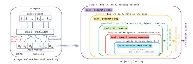
680 Figure 5. Scheme followed by SCARLET-1.0 for particle placing. On the left, the first part of the algorithm where shapes are randomly assigned to each coating particle and scaled to the actual particle size is shown. On the right, the series of five nested loops that are in charge of particle placing are presented.
