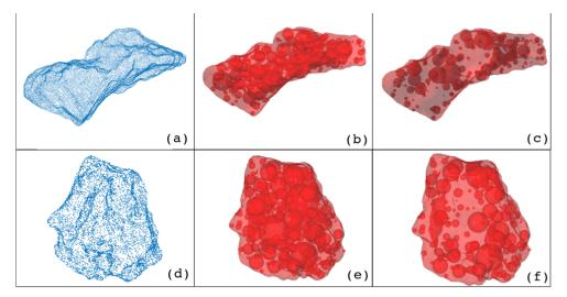
Figure 3. Application of the pre-processing routine *fromStlToSpheres* to two different volcanic particles. Blue points in (a) and (d) represent the vertices of the triangles used to define the 3D surfaces, as present in the original STL files. (b) and (e) illustrate the final process of filling the volumes with 300 spheres, placed randomly inside the objects. (c) and (f) show the most external spheres obtained using the built-in Matlab function *boundary*.
