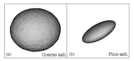
Figure 13. Ellipsoids used to characterize coarse (a) and fine (b) ash in the virtual reconstruction of the aggregates 27Sk21, 21Sk21, 22Sk20, 19Sk19 observed at Sakurajima Volcano (Japan) the 2<sup>nd</sup> and 3<sup>rd</sup> of August 2013.
