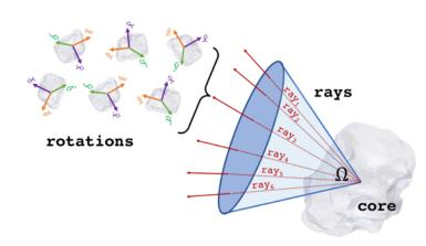
Figure 6. Cone, rays and rotations associated with the placing of one single coating particle.
