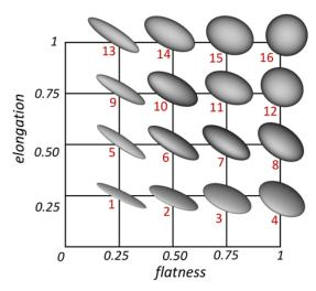
Figure 10 The *flatness-elongation plane* (FE-plane) and the associated shape of the investigated ellipsoid. The red labels in the figure are introduced to characterize each particle-particle collision univocally.
