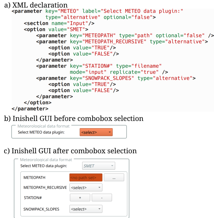
Figure 9. Example of nested widgets (for clarity, the help texts have been removed). Please note that the METEO key uses an alternate label and is defined as mandatory. Once it is selected as SMET, more widgets appear including the METEOPATH that is then also mandatory.
