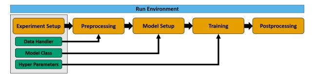
**Figure 1.** Visualization of the MLAir standard setup *DefaultWorkflow* including the stages *Experiment Setup*, *Preprocessing*, *Model Setup*, *Training*, and *Postprocessing* (all highlighted in orange) embedded in the *Run Environment* (sky blue). Each Experiment customization (bluish green) like the exemplary shown *Data Handling*, *Model Class*, and *Hyperparameter* is set during the initial *Experiment Setup* and do affect various stages of the workflow.
