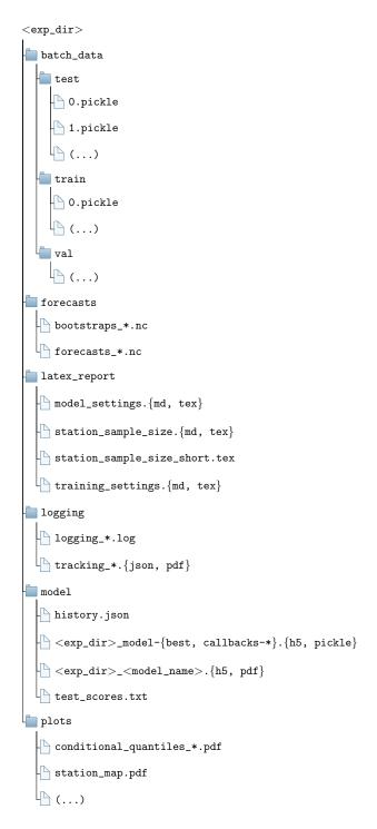
Figure 5. Default structure of each MLAir experiment with the subfolders forecasts, latex\_report, logging, model, and plots. <exp\_dir> is a placeholder for the actual name of the experiment.
