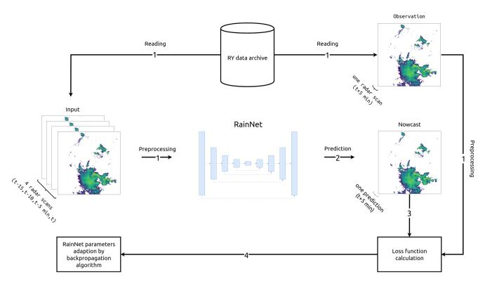
Figure 2. Illustration of one iteration step of the RainNet parameters optimization procedure.
