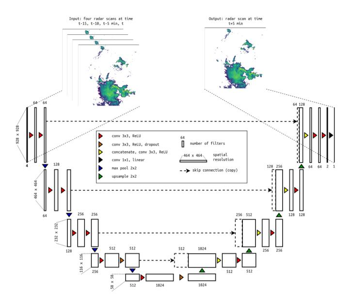
**Figure 1.** Illustration of the RainNet architecture. RainNet is a convolutional deep neural network which follows a standard encoder-decoder structure with skip connections between its branches. See main text for further explanation.
