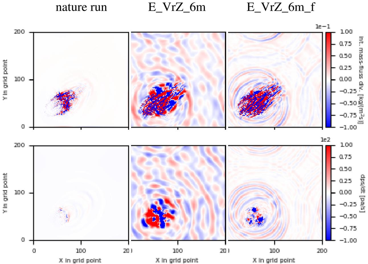
**Figure 3.** The upper row is for the integrated mass-flux divergence of nature run (left), analyses of E\_VrZ\_6m (middle) and E\_VrZ\_6m\_f (right) at 15:00 UTC; the second row is for the surface pressure tendency
