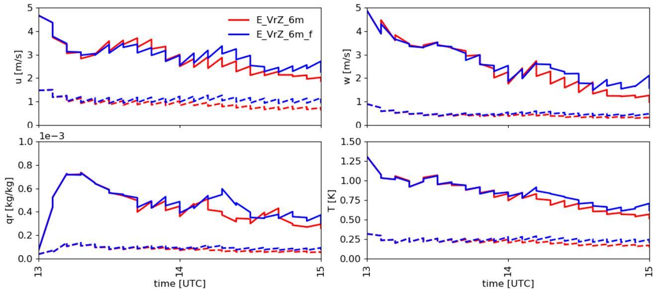
**Figure 5.** The RMSEs (solid line) and spreads (dashed line) of the deterministic background and analysis (sawtooth pattern) for  $u$ ,  $w$ ,  $q_r$  and  $T$  at each cycle in E\_VrZ\_6m and E\_VrZ\_6m\_f, averaged over points at which the reflectivity in the nature run is greater than 5 dBZ.
