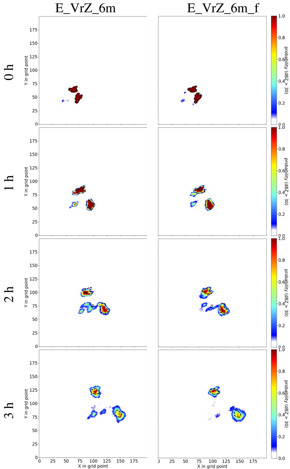
**Figure 10.** Ensemble forecasts (starting at 15:00 UTC) of E\_VrZ\_6m (left) and E\_VrZ\_6m\_f (right), based on gridpoint-based probabilities of ensemble members with reflectivity composite at elevation  $0.5^\circ$  exceeding the threshold value 30 dBZ. Reflectivity  $\geq 30$  dBZ in the nature run is denoted with contour dashed lines. The forecasts at the initial time, 1h, 2 h and 3 h are presented from top to bottom.
