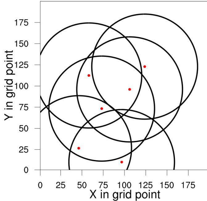
**Figure 1.** Distribution of radar network (six radars), expressed by the range of PPI (Plan Position Indicator) scan at the elevation  $0.5^\circ$
