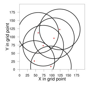
Fig. 1. Distribution of radar network (six radars), expressed by the range of PPI (Plan Position Indicator) scan at the elevation  $0.5^{-1}$
