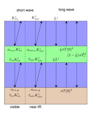
**Figure A26.** Longwave and shortwave radiation fluxes between the ground (brown), canopy (green), and overlying atmosphere. The meaning of each arrow is given at its tail. All variables are defined in the Appendix.
