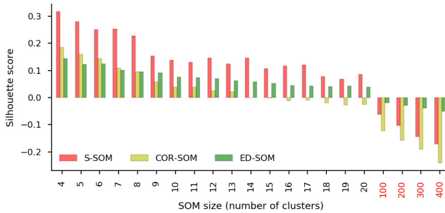
435 Fig. A10. Average silhouette scores of S-, COR- and ED-SOM. The x-axis indicates the SOM size configurations. The y-axis shows the silhouette score, which ranges from -1 to 1. For a given sample, the perfect cluster assignment has the value of 1, and negative values mean the wrong cluster assignment for the sample.
