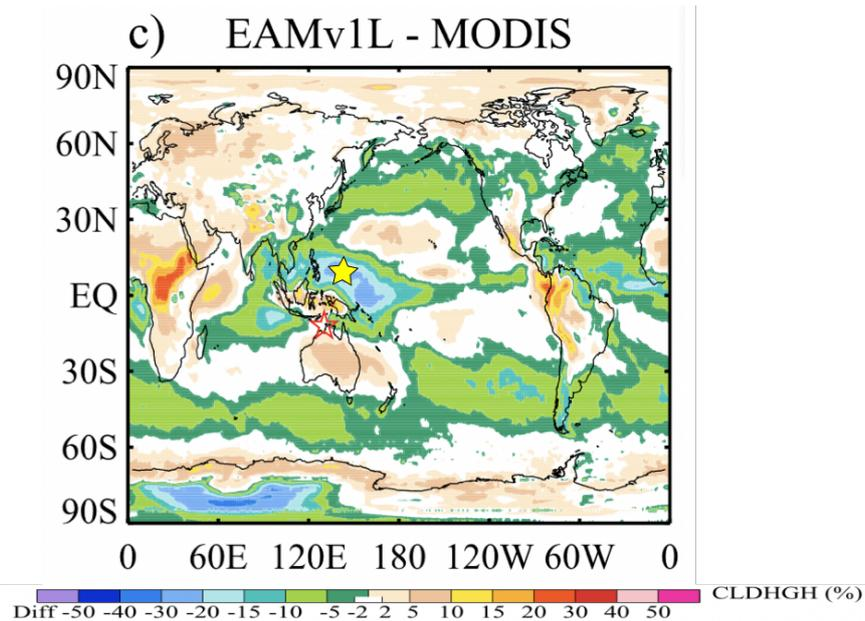
**Figure 6.** Climatological E3SMv1 high cloud bias, computed relative to MODIS observations, from Xie et al. (2018). Open red star shows location of the TWP field campaign, while solid yellow star shows the location we use for our E3SM SCM Replay experiment.
