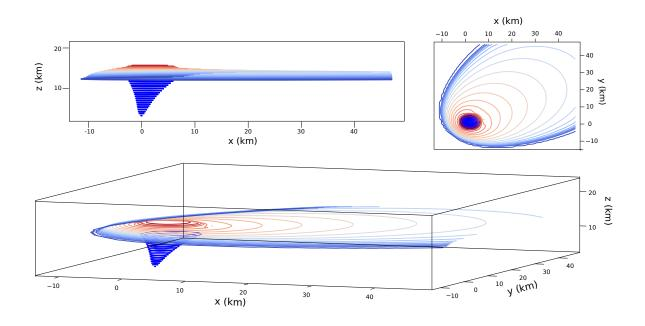
**Figure 4.** Lateral, top and oblique views of the plume and the umbrella. The 3-D coordinate system (x,y,z) is centered horizontally at the plume base location, and vertically at the sea level. Up the neutral buoyancy level the plume horizontal sections are calculated by the steady state model. Above the neutral buoyancy level, the colored contours represent thickness levels of the steady solution computed by the transient umbrella model.
