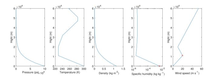
Figure 9. Atmospheric profiles for a dry atmosphere and with a 20 m s<sup>-1</sup> wind speed at the troppause (11 km asl). The red markers denote the values that can be changed in the modified standard atmosphere adopted in the model. The first three profiles (pressure, temperature and density) also change when the specific humidity at the sea level is changed.
