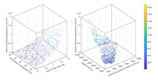
**Figure 11.** Upwind spreading of the umbrella cloud as a function of wind speed at tropopause and mass flow rate (left) and plume model output parameters (right). Please note that in the left panel also the specific humidity at sea level is varied, without producing significant variations in the upwind spreading.
