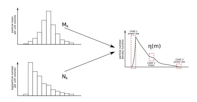
**Figure 2.** Piecewise reconstruction of the number density function from the local moments. The values of the first two moments in each section (plotted on the two bar plots on the left) are used for the reconstruction of the piecewise continuous density function. The function is linear in the internal sections and a power law at the boundaries.
