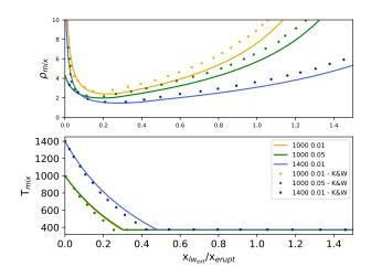
**Figure B4.** Variation of initial mixture density ( $\rho_{mix}$ ) and temperature ( $T_{mix}$ ) as the mass of water added to the magma is increased. Continuous lines show the results of PLUME-MoM, while dotted lines are digitized from Koyaguchi and Woods (1996). Curves are shown for initial magma temperatures of 1000 and 1400 K, while magma volatile content ranges from of 0.01 to 0.05 wt fraction.
