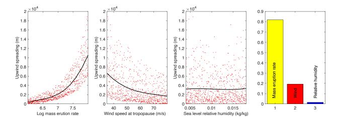
**Figure 10.** Upwind spreading of the umbrella cloud as a function of input parameters (first three panels) and main sensitivity indices (right). In the first three panels each red dot represents a different simulation, whereas the black lines represent the mean of the output parameter at a given input value. For a fixed value of the input parameters on the x-axis of a plot, the vertical spreading of the results is associated with variations in the other input parameters.
