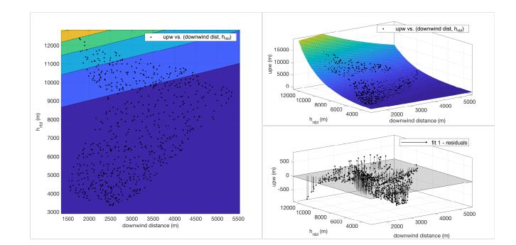
**Figure 12.** Exponential fitting of upwind spreading vs. neutral buoyancy level height and downwind displacement of the plume axis at the same height. A contour plot is shown in the left panel, while on the right a 3D view of the fitting surface (top) and the residuals of the fitting (bottom) are shown. The black dots in the left and top-right panels represent PLUME-MoM-TSM results.
