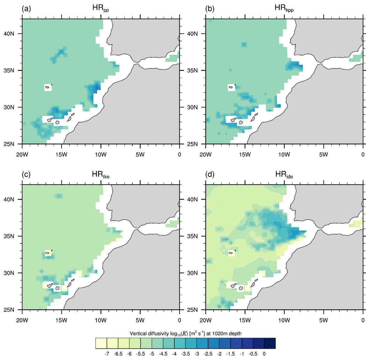
Fig 3: Vertical diffusivity  $\log_{10}(K)$  ( $m^2s^{-1}$ ) at a depth of 1020m in the Gulf of Cádiz.
