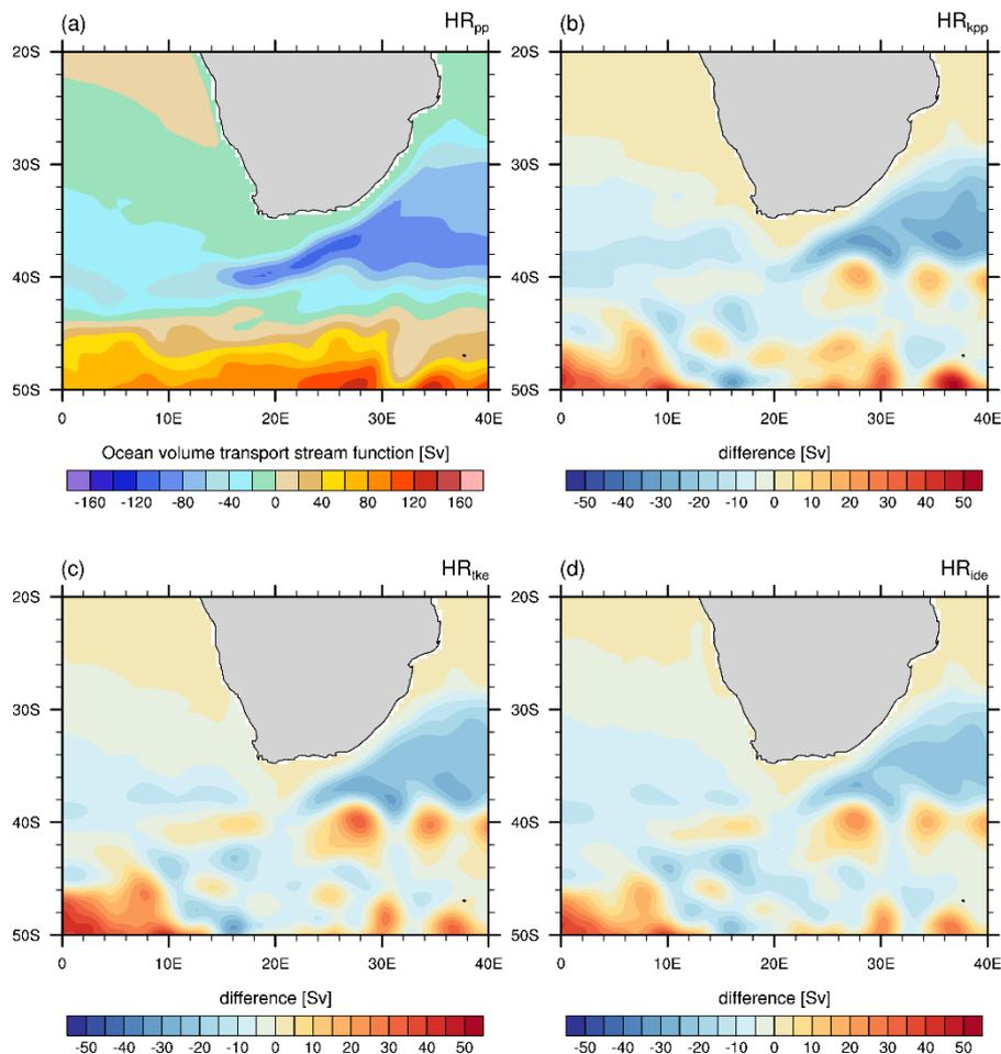
Fig. 6: Volume stream function (Sv) for the Agulhas region in (a) HRpp and the differences (experiment – HRpp) for (b) HRkpp, (c) HRTke, and (d) HRide.
