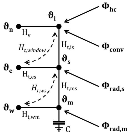
270 **Figure 1: Building indoor model: Heat flux and temperature in the R5C1 network.** The heat flux  $\Phi_w$  between  $\theta_m$  and  $\theta_w$  is calculated additionally as input value for the urban surface model, not shown in this diagram. Furthermore, the anthropogenic waste heat  $\Phi_{hc,w}$  from the heating and cooling system is calculated additionally as output value to the urban climate simulation, not shown in this diagram. (The dashed lines are for information only.)
