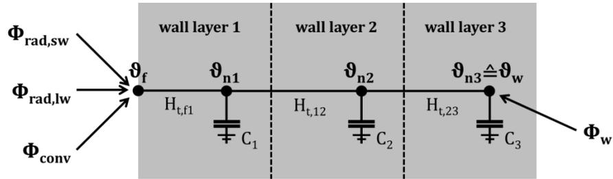
Figure 2: Urban surface model: Heat flux and temperature in the R3C3 network with three wall layers. The wall temperature  $\vartheta_w$  is the model output to the building indoor model and the heat flux into the wall  $\Phi_w$  is the input from the building indoor model, see Figure 1.
