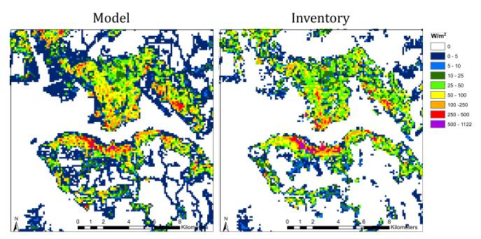
Figure 12. Anthropogenic heat flux due to building energy consumption in D5.
