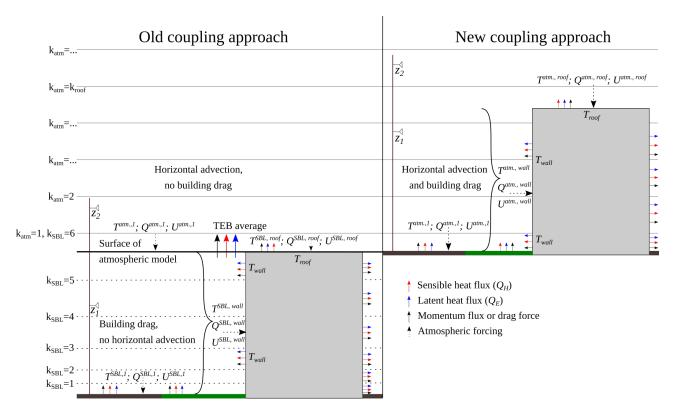
Figure 1. The old (single-layer) and new (multi-layer) approach for the coupling between Meso-NH and SURFEX-TEB. The two hypothetical wind anemometers at height above ground  $z_1$  and  $z_2$  represent at which height the model results for wind speed and direction are later compared with observations.
