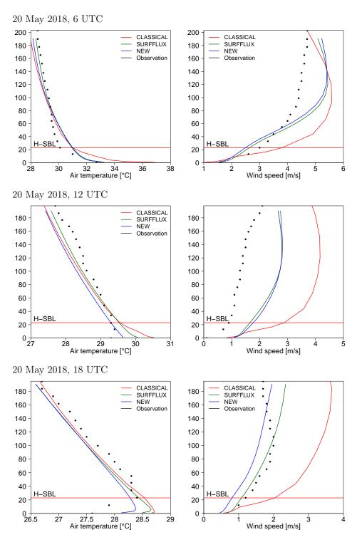
**Figure 11.** Vertical profiles of air temperature and wind speed at station King's Park. H-SBL indicates the height below which for CLASSI-CAL the meteorological variables are taken from the SBL scheme.
