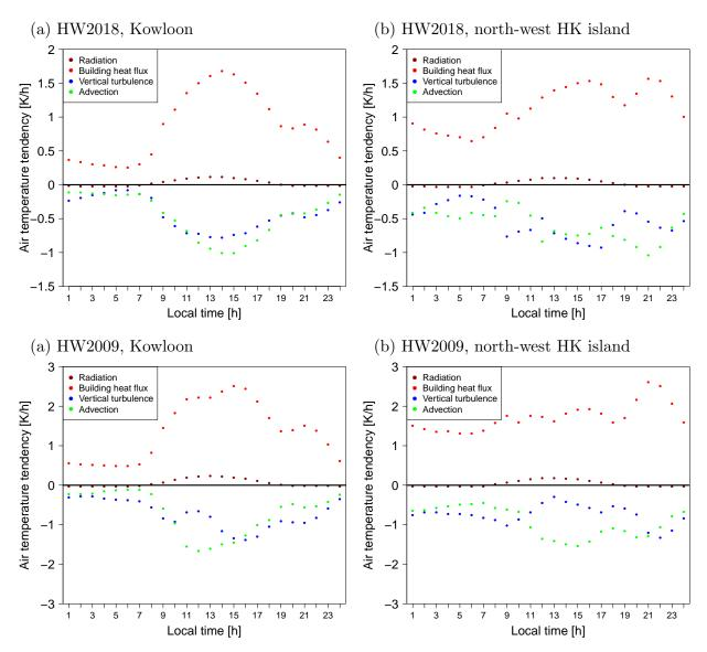
**Figure 14.** Daily cycle of the most relevant terms in the prognostic equation for the potential temperature for the NEW coupling approach in the lowest 30 m of the atmosphere for the two boxes covering Kowloon Peninsula and the north-west of Hong Kong Island displayed in Figure 10b.
