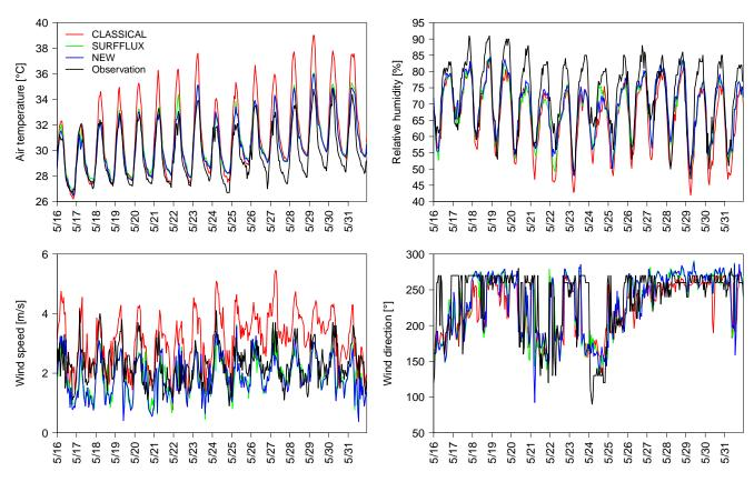
Figure 5. Time series (UTC) of simulated (D4) and observed meteorological variables at the station King's Park (KP) during HW2018.
