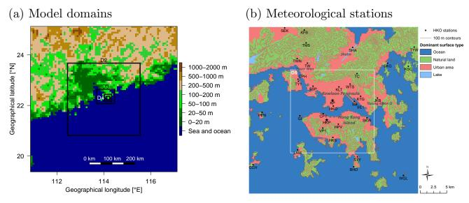
**Figure 2.** (a) The five nested Meso-NH model domains employed for the high-resolution simulation of the urban climate of Hong Kong. (b) Meteorological stations operated by the Hong Kong Observatory that are located within the model domains D4 and D5. Model results will be presented in more detail at the starred stations KP and HKP.
