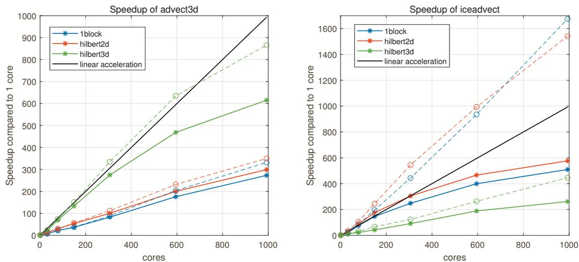
**Figure 4.** Speedup compared to one core for two functions: advect3D and iceadvect. Solid/dashed lines correspond to measurements with/without MPI-exchanges, respectively. Different partitions are shown in colour (1block, hilbert2d, and hilbert3d).
