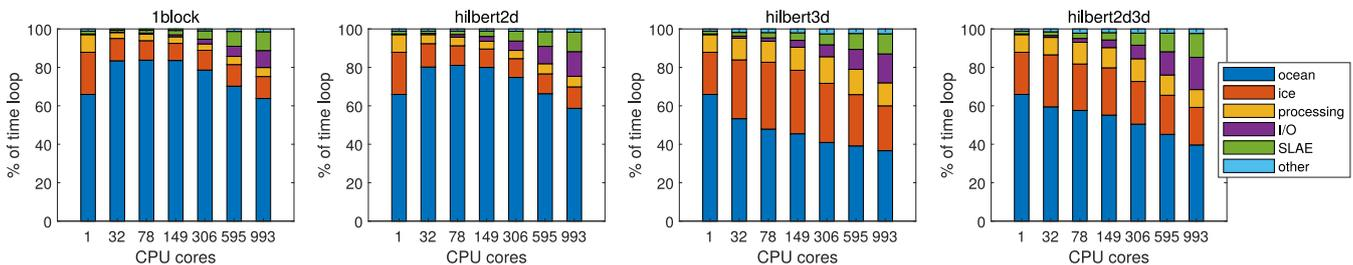
**Figure 8.** Relative contribution of different code sections to runtime; "ocean" – all procedures corresponding to ocean submodel including `advect3D`, "ice" – ice submodel including `iceadvect`, "processing" – computation of statistics, "I/O" – input/output with scatter-gather functions; "SLAE" – matrix inverse and RHS preparation; "other" – simple service procedures.
