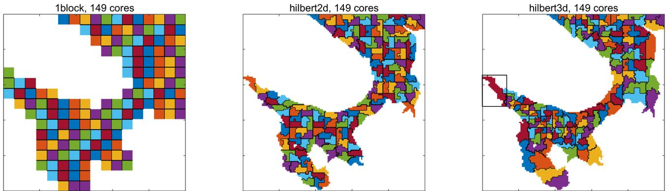
**Figure 2.** Three types of partition. Different processor cores are separated by a black line. Hilbert partitions are based on a grid of  $n_b \times n_b = 128 \times 128$  blocks. Colours can repeat. Black rectangle corresponds to a "shared" array allocated for blocks belonging to a given CPU core.
