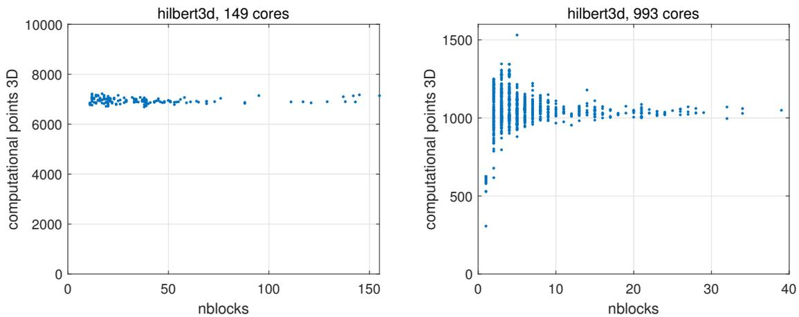
**Figure 6.** Scatter plot: number of blocks on a core – number of computational points for 3D calculations. Each point corresponds to one CPU core. Figures correspond to hilbert3d partition with different numbers of CPU cores.
