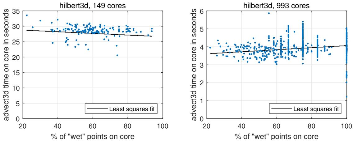
**Figure 5.** Scatter plot: percentage of wet points on a core – advect3D runtime (without MPI exchanges, for 1 model day). Each point corresponds to one CPU core. Figures correspond to hilbert3d partition with different numbers of CPU cores.
