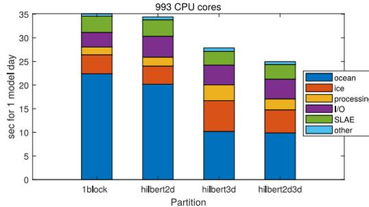
**Figure 9.** Absolute contribution of different code sections to runtime on 993 CPU cores.
