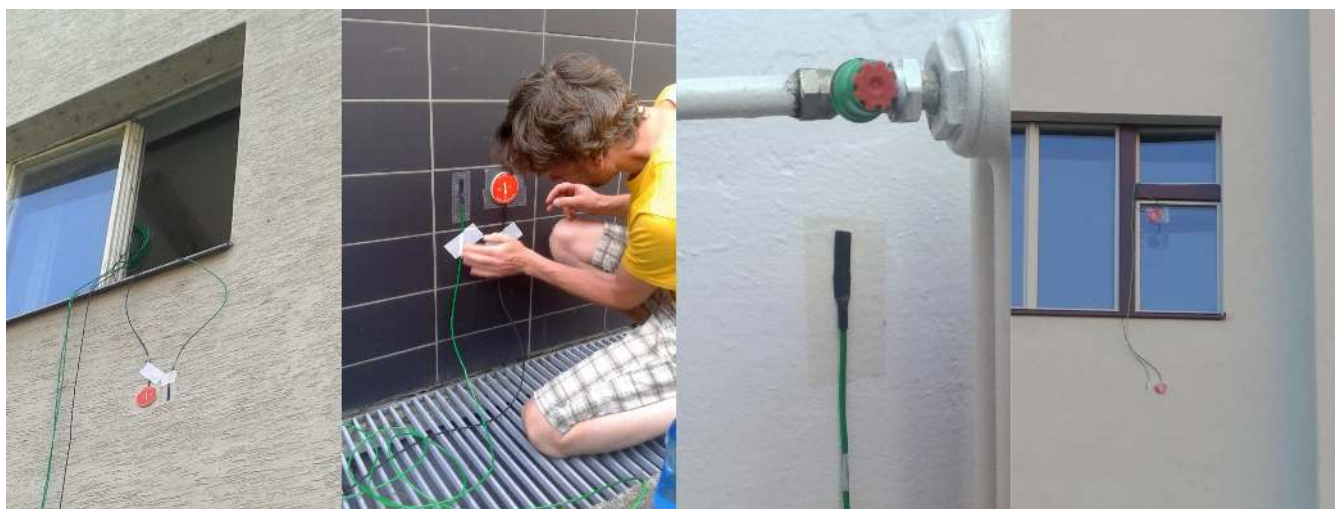
Figure 2. Detail of heat flux sensors sensor and thermocouples thermocouple mounting. Left - Sinkule house 1 st floor; center-left - Sinkule house ground floor; center-right - Sinkule ground floor - inner temperature sensor; right - Zelená Street. For Sinkule house and Zelená Street location locations see Fig. 1.
