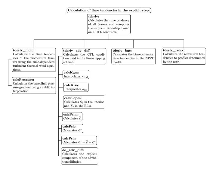
Figure 4. The call tree from the main function of mamebus.c
