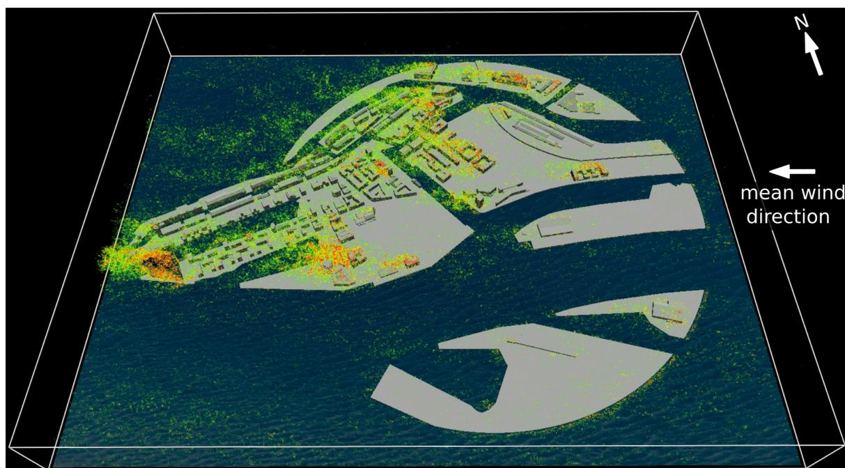
**Figure 7.** View of the volume-rendered instantaneous turbulence structures above the building array. Turbulence is visualized using the magnitude of the rotation of the velocity field. Green and red colour show low and high values, respectively. Image was rendered using VAPOR (Li et al., 2019).
