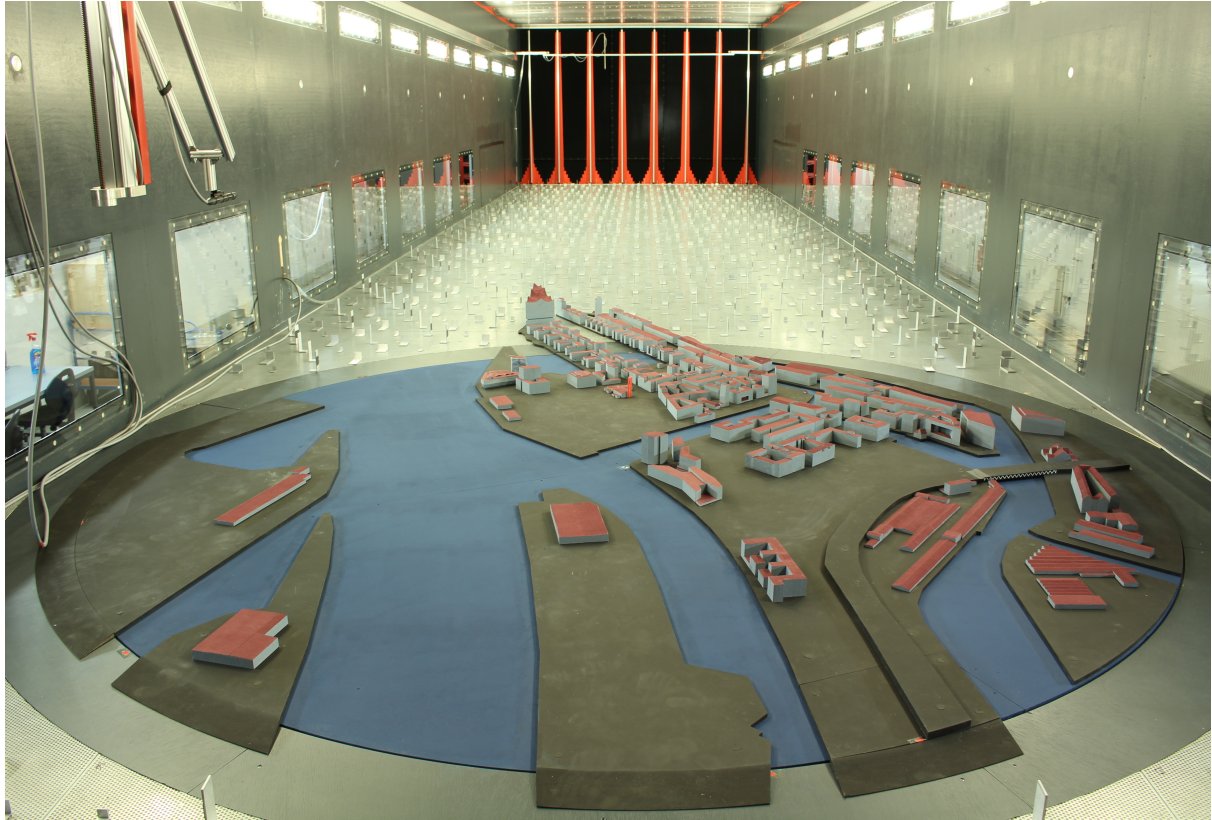
Figure 1. Photograph of the building setup within the wind-tunnel facility 'WOTAN' for an approaching flow of 290^\circ . Please note that contrary to the depicted orientation, an approaching flow from 110^\circ was used within this study.
