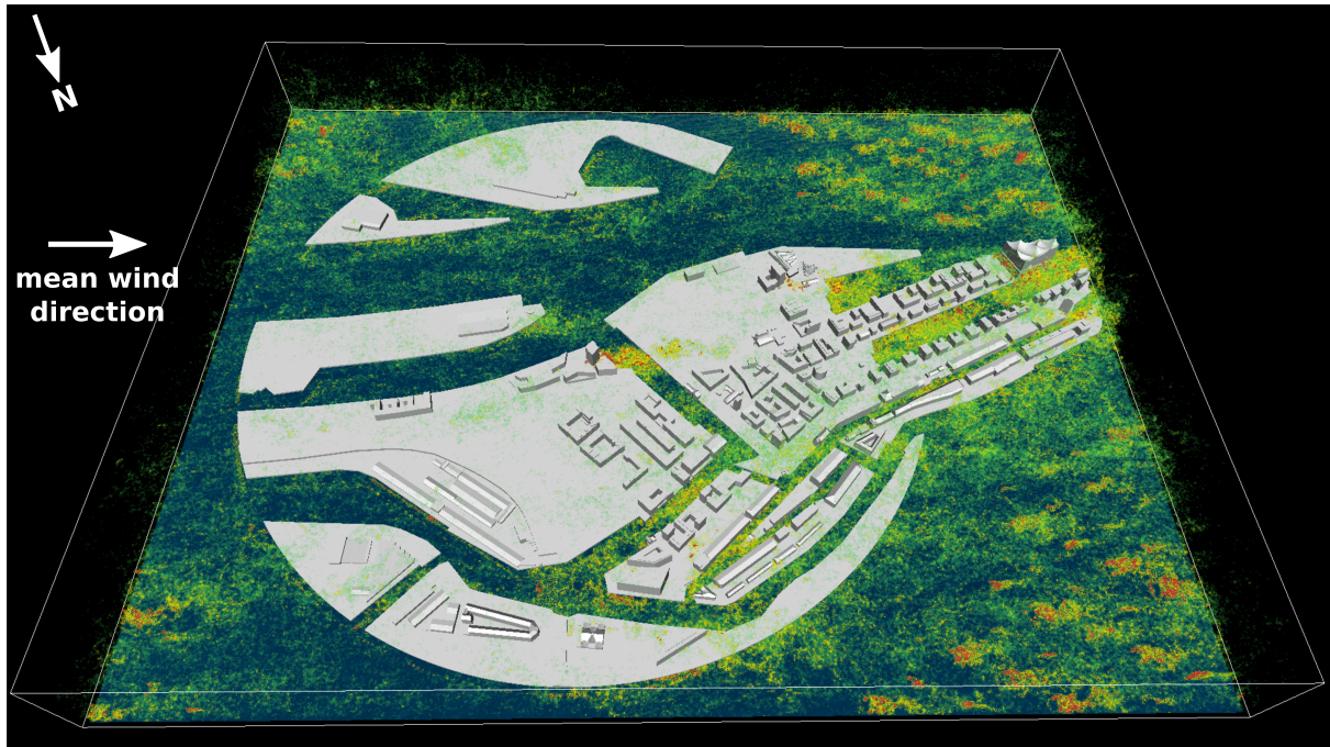
Figure 7. View of the volume-rendered instantaneous turbulence structures above the building array. Turbulence is visualized using the magnitude of the three-dimensional vorticity. Green and red colour show low and high values, respectively. Image was rendered using VAPOR (Li et al., 2019, www.vapor.ucar.edu ), the background image was designed by freepic.diller / Freepik ( http://www.freepik.com ).
