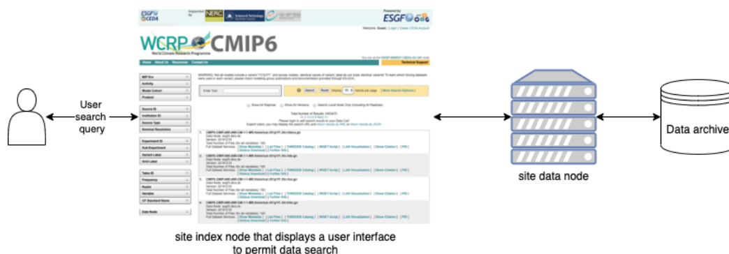
Figure 3. The ESGF data search and delivery system schematic.
