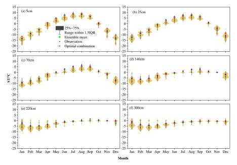
**Figure 2.** Monthly soil temperature (ST) at (a) 5 cm, (b) 25 cm, (c) 70 cm, (d) 140 cm, (e) 220 cm, (f) 300 cm at TGL site. Limits of the boxes represent upper and lower quartiles, whiskers extend to 1.5 times the interquartile range (IQR). The green circles in the box are the ensemble mean values. The light orange shading represents the kernel density distribution of simulated ST. The red diamonds are observations and the blue circles are the results of the optimal scheme combination.
