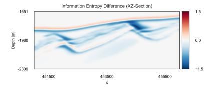
Figure 11. XZ-Section of entropy difference between the forward simulated entropy and the approximate posterior entropy H ( $\epsilon = 0.025$ ). The plot highlights areas where the entropy was reduced (blue), increased (red) and kept constant (white).
