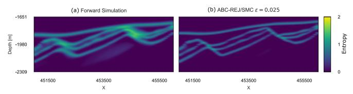
Figure 10. (a) Section of the entropy block of the forward simulation for the prior uncertainty ( $H_T = 0.223$ ); (b) Section of the entropy block of the final epoch ( $\epsilon = 0.025$ ) of the ABC-SMC simulation ( $H_T = 0.113$ ).
