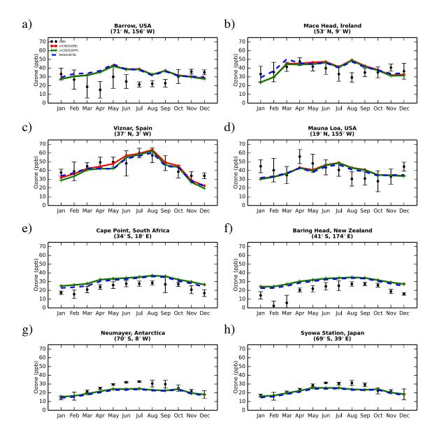
Figure 5: Monthly mean comparison of TM5-MP surface  $O_3$  (ppb) against surface observations (black line) from EMEP and WOUDC databases for the two chemistry schemes, mCB05(KPP) (green line) and MOGUNTIA (blue line), using co-located model output for 2006 sampled at the measurement times; error bars indicate the standard deviation in the monthly means. For comparison, model results of the mCB05 with the EBI solver (red line) are also presented.
