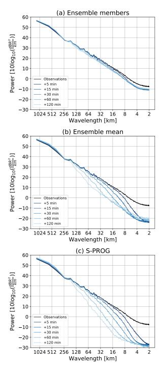
**Figure 9.** Spatial structure analysis of a) stochastic ensemble members, b) ensemble mean, and c) S-PROG filtering. To be comparable, the incremental mask and probability matching were used for both the ensemble mean and S-PROG nowcasts. All nowcasts used the Lucas-Kanade optical flow on the same event of Fig. 8. The ensemble is composed of 48 members. All models used a cascade of 8 levels without motion perturbations.
