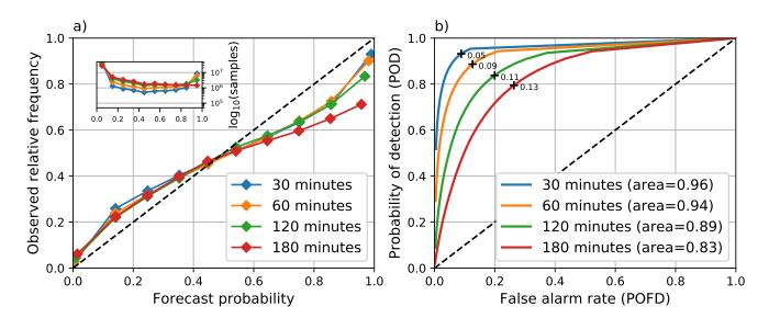
**Figure 5.** Reliability diagrams (a) and ROC curves (b) computed from STEPS nowcasts during the MeteoSwiss events listed in Table 8 with different lead times and threshold  $0.1 \text{ mm h}^{-1}$ . The default settings listed in Table 5 were used for computing the nowcasts. The optimal probability thresholds that maximize POD-POFD are marked in the ROC curves with black crosses.
