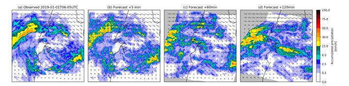
**Figure 20.** Comparison of a member of 5-min rainfall ensemble for (b) +30 minutes, (c) +60 minutes and (d) +120 minutes nowcasts initialized with (a) radar-based rainfall analysis from the Australian radar network valid at time 0605 UTC 01 January 2019 on a 512x512 pixel grid (256x256 km) (event no. 2 in Table 10).
