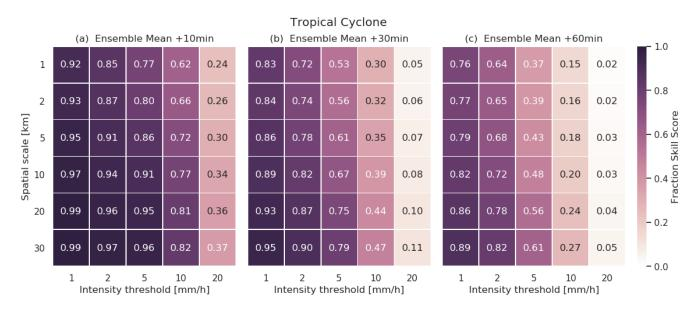
**Figure 22.** Comparison of Fractions Skill Score (FSS) values for (a) +10 minutes, (b) +30 minutes and (c) +60 minutes nowcasts rainfall ensembles for Tropical Cyclone Penny (event no. 1 in Table 10). FSS values were calculated comparing the ensemble mean for each lead time with observations.
