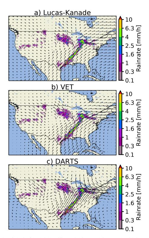
**Figure 12.** Comparison of advection fields obtained by different optical flow methods for a selected precipitation event: US, 2013/04/11 0800 UTC.
