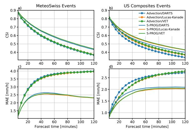
**Figure 11.** Comparison of forecast skill using different optical flow and extrapolation methods. The left panel shows the averaged CSI and MAE for the MeteoSwiss events listed in Table 8, while the right panel shows the same results but for the US events listed in Table 9.
