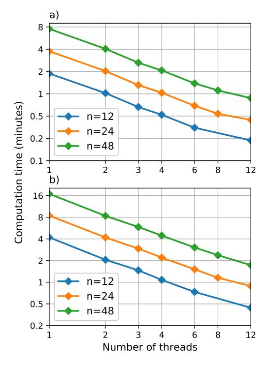
**Figure 15.** Averaged computation times of pysteps nowcast ensembles with different ensemble sizes and number of parallel threads for the (a) MeteoSwiss and (b) FMI domain. The grid sizes for the domains are 710x640 and 760x1226 pixels, respectively. One-hour nowcasts with 12 time steps of 5 minutes were computed for both domains. The computation times include only the ensemble computation, excluding the optical flow, the initialization of the model and writing the results to disk.
