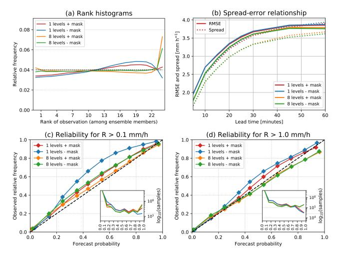
**Figure 19.** Ensemble and probabilistic verification of the cascade experiments for all the MeteoSwiss cases with and without cascade decomposition, and with and without masking. a) Rank histograms at 60 min, b) spread-error relationship, c,d) reliability diagrams at 60 min for probability of rain exceeding 0.1 and 1 mm  $h^{-1}$  respectively.
