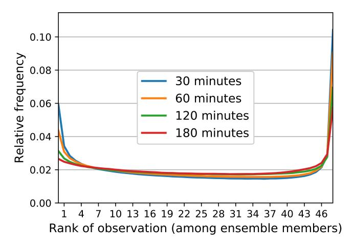
**Figure 7.** Rank histograms computed from STEPS nowcasts during the MeteoSwiss events listed in Table 8 with different lead times. The default settings listed in Table 5 were used for computing the nowcasts.
