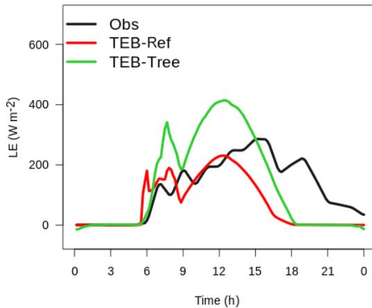
**Figure 4.** Comparison of the TEB-Ref and TEB-Tree results (red and green lines, respectively) with the latent heat flux deduced from measurements of tree transpiration and grass evaporation (black line).
