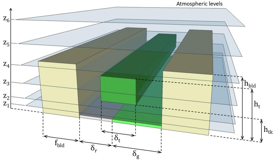
**Figure 1.** Schematic representation of the TEB urban canyon, integrating a part of ground-based natural covers and an explicit tree-foilage layer, and of the atmospheric vertical levels of the surface boundary layer (SBL) scheme coupled to TEB to compute vertical profiles of micrometeorological variables inside and above the canyon.
