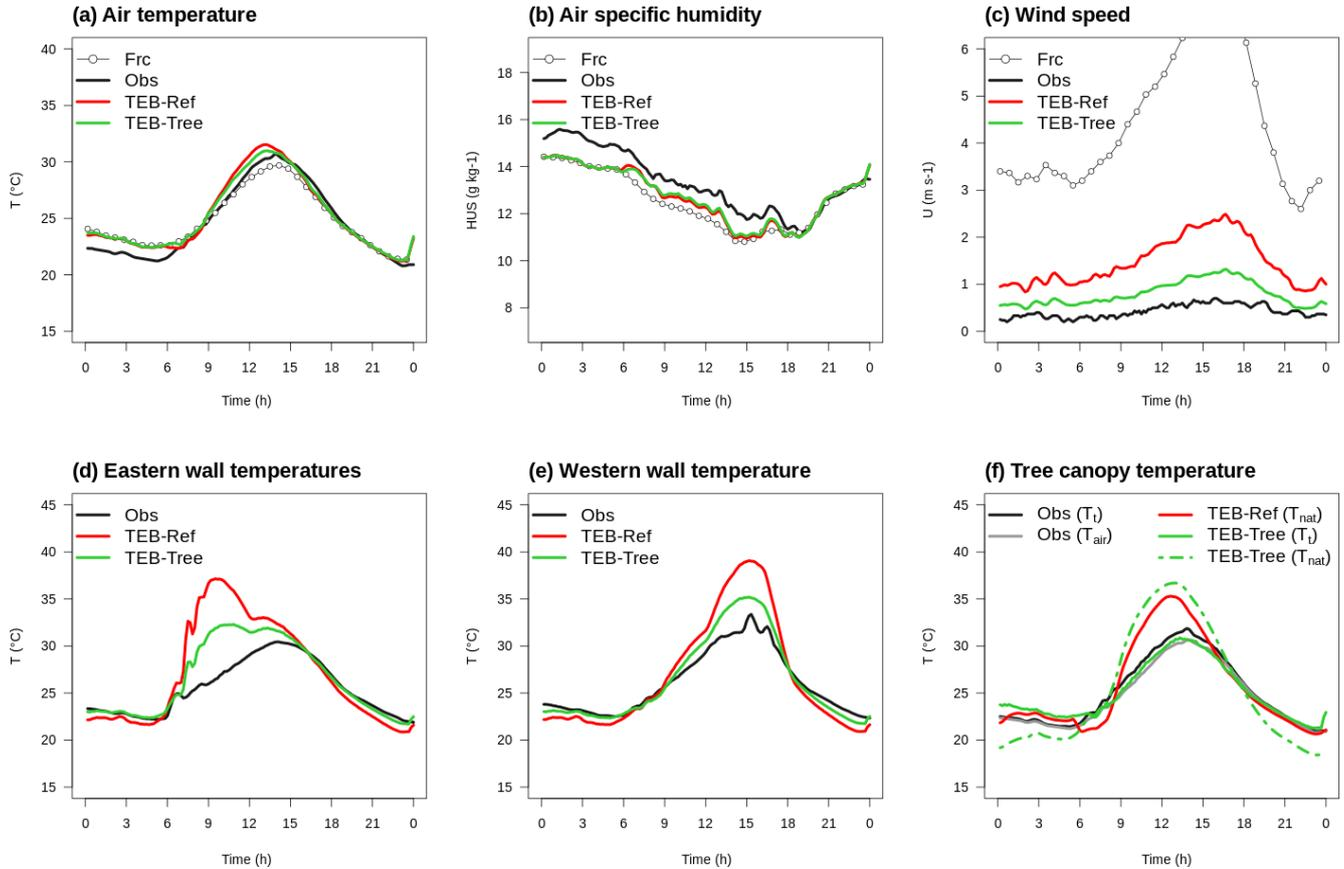
**Figure 3.** Comparison of the TEB-Ref and TEB-Tree results (red and green lines, respectively) with meteorological variables (a–c) and surface temperatures of urban facets and trees (d–f) measured within the courtyard (black line). For air temperature, specific humidity and wind speed, the gray line with symbols indicates the forcing data above the buildings.
