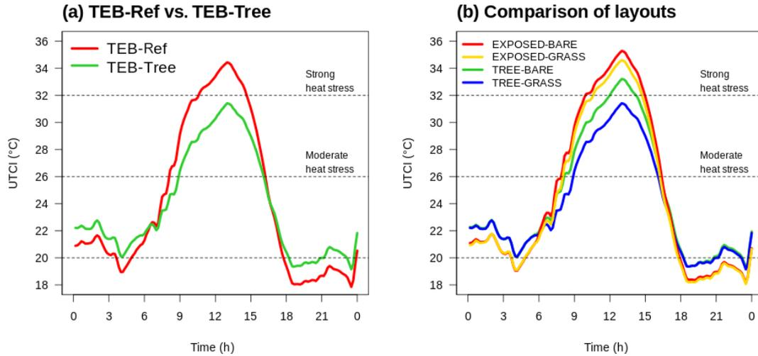
**Figure 5.** (a) Comparison of UTCI simulated in the courtyard by TEB-Ref (red line) and TEB-Tree (green line) for TREE-GRASS configuration; (b) comparison of UTCIs simulated by TEB-Tree for four different courtyard layouts.
