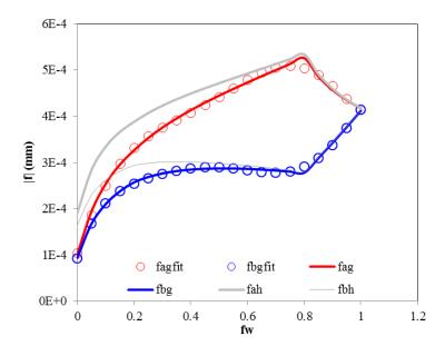
The backscatter amplitudes of hail are shown with gray solid lines; they are higher than their graupel counterparts (red for fa and blue for fb) as reviewer mentioned. Circles are fitting results using our graupel coefficients. These new coefficients are listed in Tables 1 and 2 in the revision.
