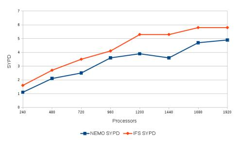
Figure 1 NEMO (red) and IFS (blue) scalability in EC-Earth3P-HR. The throughput is expressed in simulated years per day (SYPD) of wall clock time. The tests have been performed on the MareNostrum4 computer at the Barcelona Computing Centre with full output and samples of five one-month runs for each processor combination, the average of which is shown in the figure. The horizontal axis corresponds to the number of cores used.
