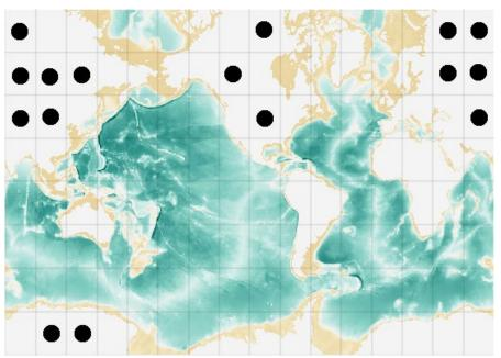
920 Figure 4 Domain decomposition of a tripolar grid of the ORCA family with a resolution of a of degree into 128 subdomains (16 x 8). Subdomains marked with a black dot do not contain any ocean grid point.
