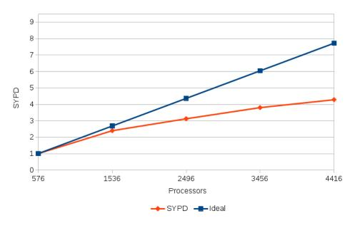
**Figure 2** As Fig. 1 but now for the scalability of the fully coupled EC-Earth3P-HR. The blue diagonal indicates perfect scalability.
