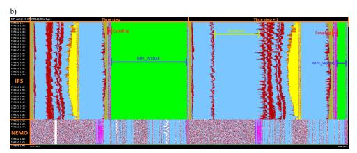
**Figure 3** (a) Paraver view of the NEMO and IFS components in an EC-Earth3P-HR model execution for two time steps including the coupling process. The horizontal lines give the behaviour of the different processes (1 to 512 for IFS and 513 to 536 for NEMO) as a function of time. Each colour corresponds to a different MPI communication function. See text for explanation. (b) as (a), but now when optimization options "opt" and "gathering" for coupling are activated.
