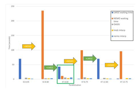
**Figure A2.** Waiting time of the model components and computation time of the coupler and interpolations, as a function of incremental resources provided to each component. The XX.X.X code on the x-axis indicates successively the number of MPI processes, OMP threads for LMDZ and MPI processes for NEMO. This shows that most efficient configuration is the one with 47 MPI and 8 OMP dedicated to LMDZ and 60 MPI dedicated to NEMO.
