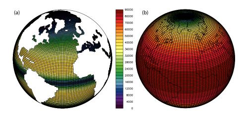
**Figure 1.** NEMO (a) and LMDZ (b) grid cell areas, in km<sup>2</sup>, showing the refinements of the ocean grid in the tropics and over the Mediterranean Sea as well as the refinement of the atmospheric grid to the pole.
