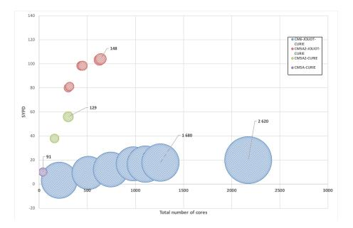
Figure A10. Scalability, i.e. SYPD as a function of parallelization, of IPSL-CM5A2 on CURIE and JOLIOT-CURIE supercomputers compared to IPSL-CM6-LR (blue disks) on JOLIOT-CURIE. The surface of the disks is proportional to the computing cost (CHSY).
