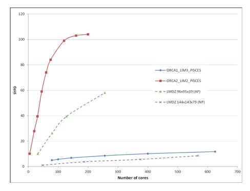
Figure A1. Computing performances for LMDZ and NEMO component at two resolutions in the early tests made on supercomputer CURIE.
