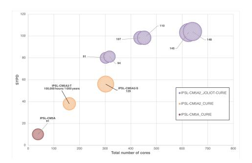
**Figure 2.** Scalability, i.e. SYPD as a function of parallelization, of IPSL-CM5A2 on CURIE and JOLIOT-CURIE supercomputers. The surface of the disks is proportional to the computing cost (CHSY).
