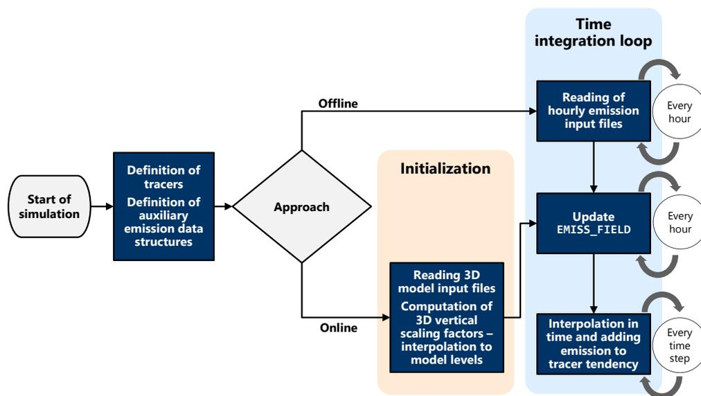
**Figure 2.** Flow chart for COSMO-GHG run-time processes both for the offline and online approach.
