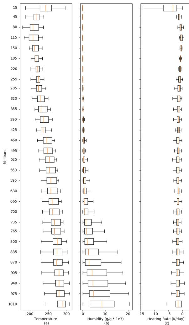
**Figure 1.** (a,b) ERA-Interim air temperature (K) and humidity ( $\text{g kg}^{-1}$ ) statistics. (c) Longwave radiative rates ( $\text{K day}^{-1}$ ) calculated using RRTMG. Vertical axis is pressure in Pa.
