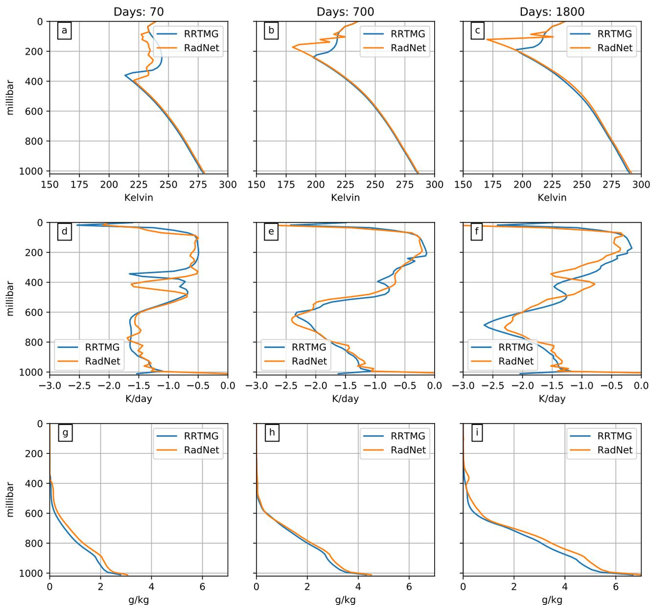
**Figure 6.** Comparison of the vertical profiles of temperature (first row), longwave heating rates (second row) and specific humidity (third row) for the RadNet and RRTMG simulations at three different times.
