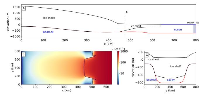
Figure 2. Initial ice-sheet in equilibrium calculated by Elmer/Ice with an accumulation rate of  $0.3 \ m \ a^{-1}$  and no sub-shelf melting as required by the MISMIP+ protocol (Asay-Davis et al., 2016). (A) Side-view geometry in the central flowline, also indicating the position of the ocean restoring used by the ocean model. (B) Velocity magnitude seen from above. The black solid line indicates the grounding line. (C) Cross section of the ice sheet at  $x = 480 \ km$ .
