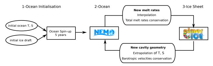
Figure 1. NEMO-Elmer/Ice coupling framework. T and S stand for temperature and salinity.
