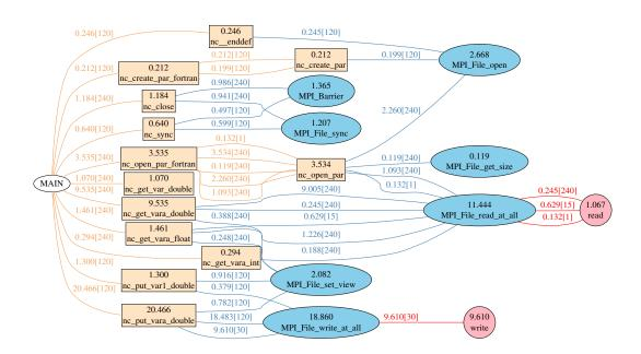
Figure 12. The callpath flow of tuned 240-PE benchmark with PnetCDF.
