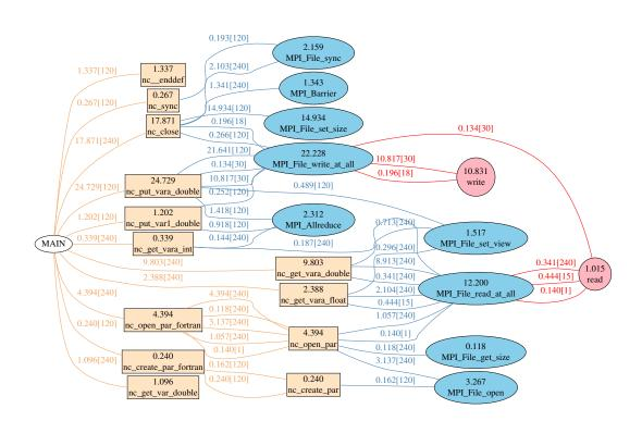
Figure 11. The call path flow of tuned 240-PE benchmark with HDF5 1.10.2/netCDF-4.
