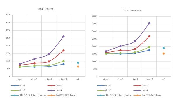
Figure 15. Performance of 720-PE runs with customized chunk layouts in HDF5/netCDF-4. The default chunk layout of HDF5/netCDF-4 and contiguous layout of PnetCDF/netCDF-3 are shown as references.
