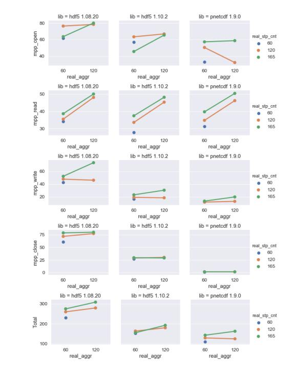
Figure 9. The I/O performance of different library/format bindings with a variety of aggregators and stripe counts by using 960 PEs.
