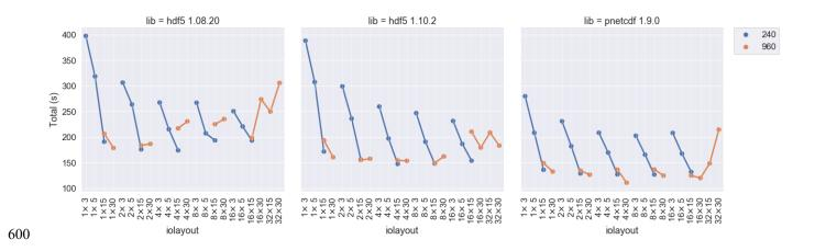
Figure 7. Total elapsed time versus I/O layout for different libraries and formats. Higher contention at 960 PEs can overwhelm the overall performance trends observed at 240 PEs.
