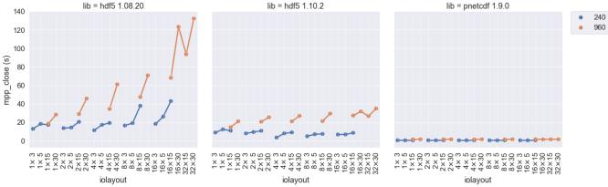
595 Figure 6. mpp\_close time versus I/O layout with different libraries and formats. Contentions within the HDF5 library lead to performance problems, which increase with layout and number of PEs. PnetCDF does not exhibit these issues and close times are negligible.
