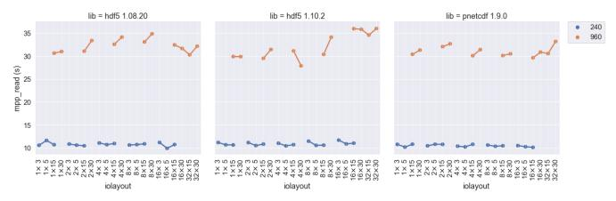
585 Figure 4. mpp\_read time (in sec.) versus I/O layout in different libraries and PE numbers. Read operations do not use I/O layout or parallel I/O, and runtimes are largely independent of layout and library. Read times increase significantly as the number of PEs is increased.
