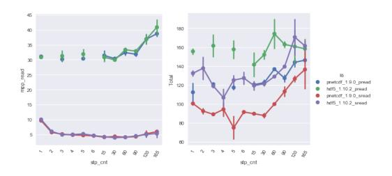
650 Figure 14. The 960-PE benchmarks with an I/O layout of 4×30 and using serial read (sread) and parallel read (pread) with the HDF5 1.10.2 and PnetCDF libraries. Serial read times are overall more efficient over a range of stripe counts.
