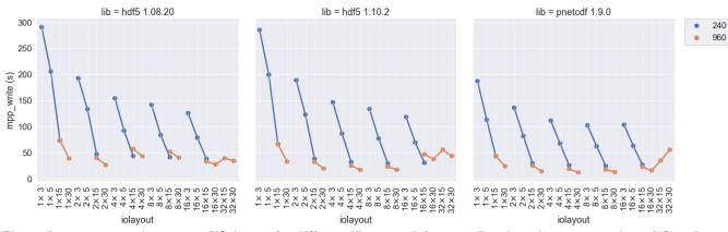
Figure 5. mpp\_write time versus I/O layout for different library and formats. Runtimes improve greatly as I/O nodes are increased (grouped curves), and modestly as the I/O PEs per node are increased (across grouped curves). Runtimes are scalably reduced as PEs are increased. PnetCDF shows modest improvement over HDF5 performance.
