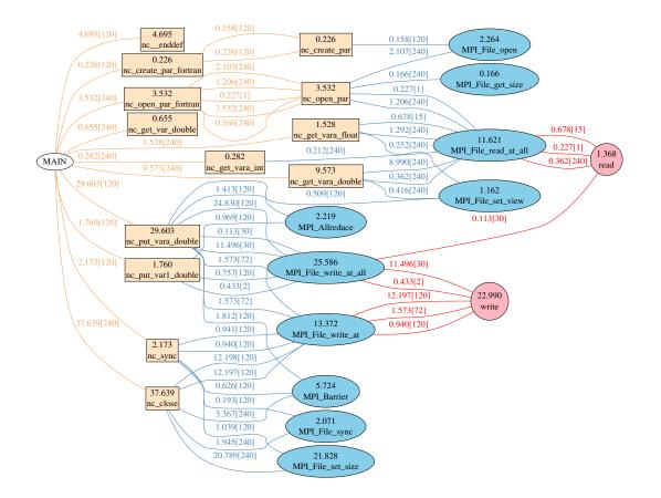
Figure 10. The call path flow of a tuned 240-PE benchmark with HDF5 1.8.20/netCDF-4. It is classified into 3 layers i.e. netCDF, MPI-IO and system I/O functions. The maximum PE time together with the total number of PEs from the invoker are labelled above each path line and the maximum PE time on each function are labelled within the node block.
