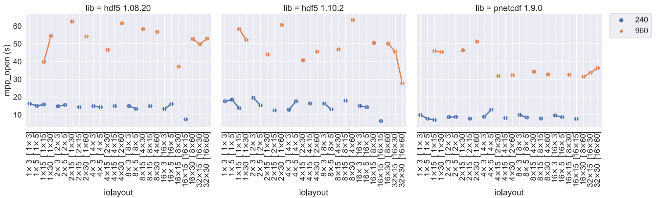
625 Figure 3. mpp_open time (in sec.) versus I/O layout in different libraries and PE numbers. HDF5 times are generally larger than in PnetCDF, and the runtime increases as PEs increase from 240 to 960. The I/O layout together with its PE distribution in [PE per node × nodes] are labelled in X-axis.
