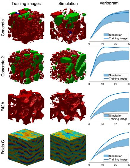
626 Figure A 3 Examples of 3D simulation results
