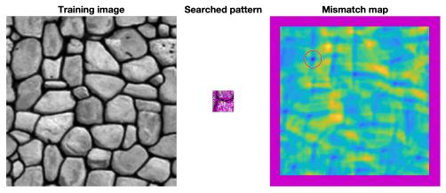
Figure 1 Example of a mismatch map for an incomplete pattern. Blue represents good matches and yellow bad matches. The red circle highlights the minimum of the mismatch map, which corresponds to the location of the best candidate.
