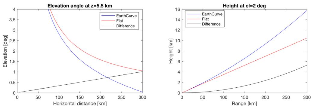
Figure 1: (Left) Elevation angle at a fixed height of 5.5 km AGL as a function of horizontal distance from the curved surface including the atmospheric refraction (blue) and flat surface (red) assumptions. (Right) Height at a fixed elevation angle of  $2^\circ$  as a function of radar range. Black lines represent the difference between the two assumptions. The curved surface is assumed to be a sphere surface with a radius of 6370.0 km.
