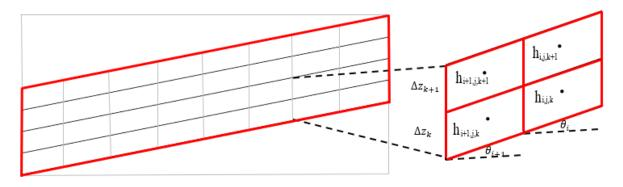
Figure 2: Representation of orthogonal (upper) and the terrain following (lower) grid formulations and schematics of the associated finite difference dependences (right). The i, j, and k are the x, y, and z cell indices
