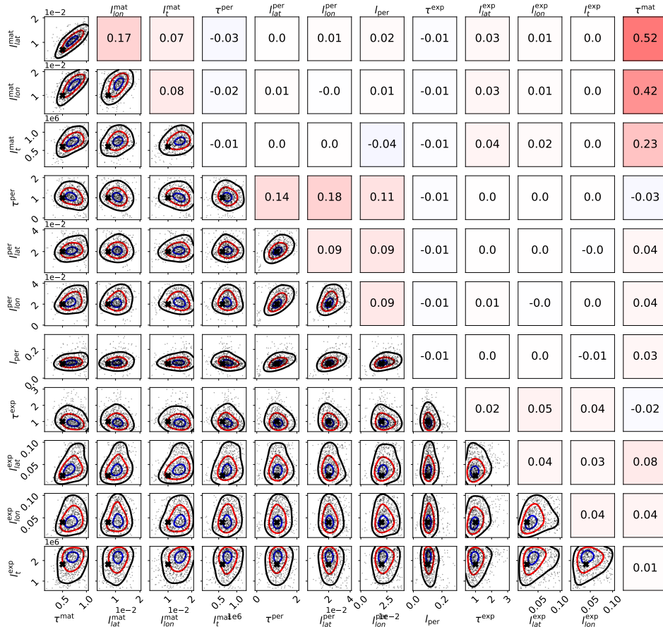
Figure 16. Scaled MCMC posteriors from a synthetic study where data was generated with a multi-scale Gaussian process. The figure demonstrates that even with three subkernels, multi-scale Gaussian process kernel parameters can be recovered. The lower left part shows the pairwise marginal distributions of the parameters, and the black crosses denote the true parameter values. The axis labels are on the left and below the figure. The upper right triangle shows sample correlations between the parameters from the chain, with axis labels on the left and on the top. Small within-subkernel positive correlations are present. The contours shown include 85% (black), 50% (red), and 15% (blue) of the posterior mass.
