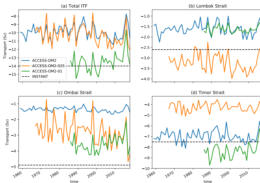
Figure 18. Timeseries of annual-mean transport through the Indonesian Straits. The total Indonesian Throughflow (panel a) can be broken into (b) Lombok Strait; (c) Ombai Strait and (d) Timor Strait. Black dashed lines indicate the mean throughflow during 2004–2006 from the INSTANT program (Sprintall et al., 2009). Negative values indicate southward flow.
