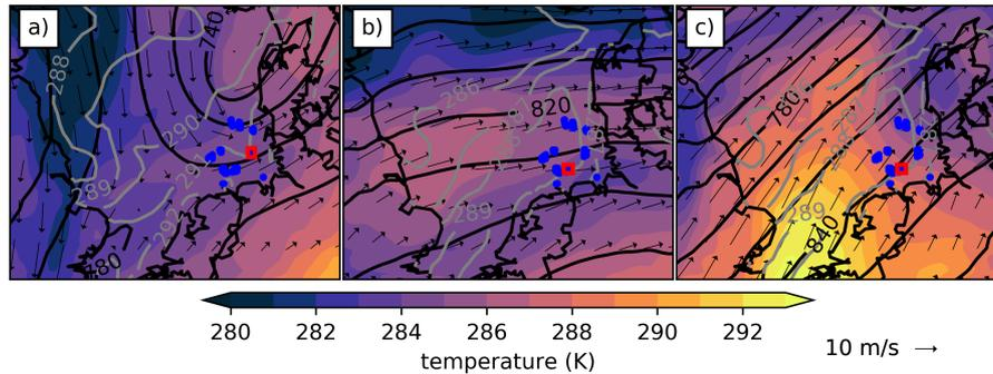
**Figure 5.** ERA5 reanalysis data: Temperature (colored contours (K)) and geopotential height (20-m increments) as black contour lines in 925 hPa for the three case studies as listed at Table 1, at 15:00 UTC 09 August 2017, at 15:00 UTC 14 October 2017 and at 09:00 UTC 15 October 2017 (Table 1). The gray solid contour lines show the SST.
