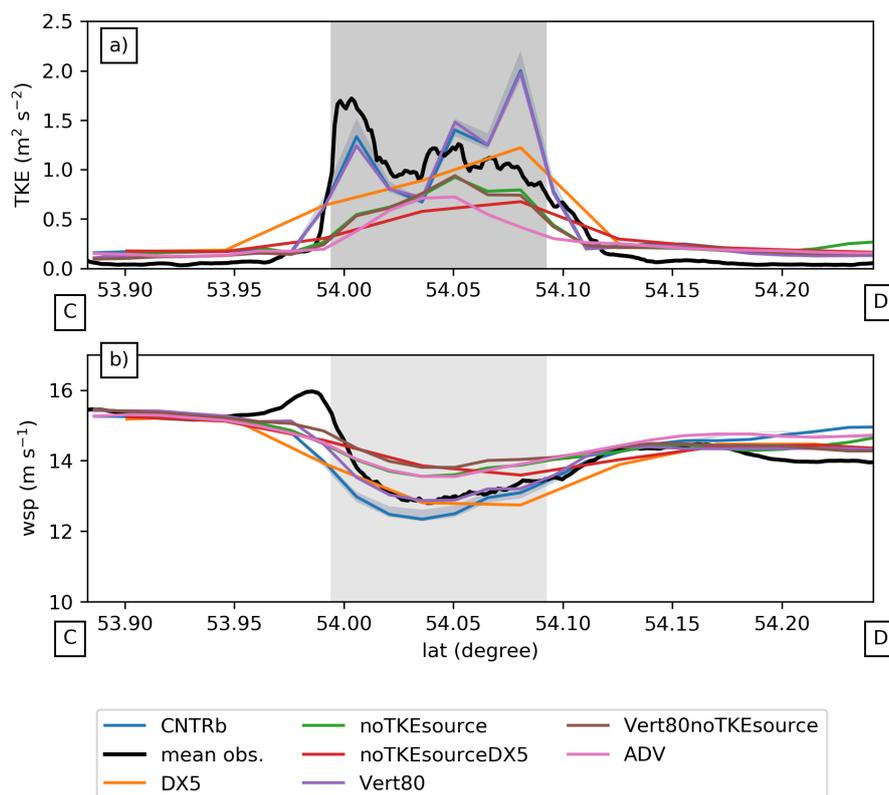
**Figure 12.** As in Fig. 8, but for TKE (a) and wind speed (b) for the sensitivity simulations DX5, noTKESource, DX5noTKESource, Vert80, Vert80noTKESource and ADV conducted for case study II. For better comparison the control simulation CNTRb plotted as well.
