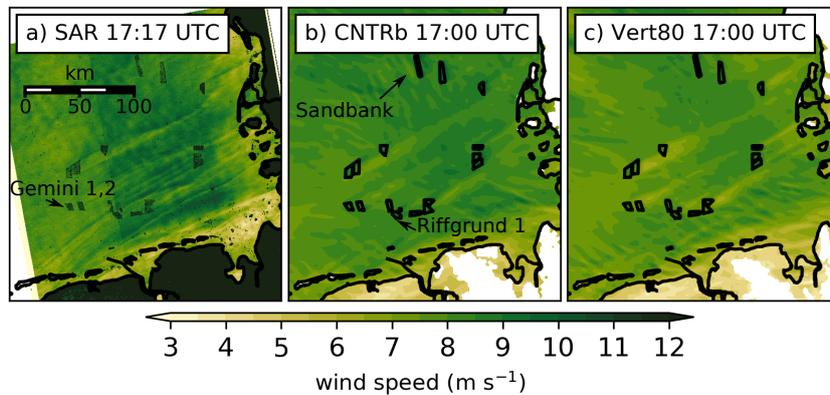
**Figure 4.** A comparison of SAR from Copernicus Sentinel 1A and WRF retrieved wind speed at 17:17 UTC and 17:00 UTC, respectively, on 14 October 2017 (case study II). The SAR data shows the wind speed at 10 m, whereas the model output is taken from the model level closest to 10 m. Therefore, we show the wind speed in 17 m and in 15 m for the CNTR and Vert80 simulation, respectively.
