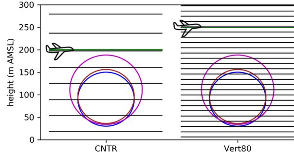
**Figure 3.** Distribution of the vertical levels with height and the levels intersecting with the rotor areas of the two wind turbine types used in the wind farms as listed in Table 3 for the CNTR and the Vert80 simulation. The rotor areas of the wind turbines SIEMENS-SWT-6.0-154, SIEMENS SWT 3.6-120 and SENVION 6.2 is shown in magenta, blue and red, respectively. The green lines denote flight heights at 200 m and 250 m AMSL; necessary due to the two different wind turbine types.
