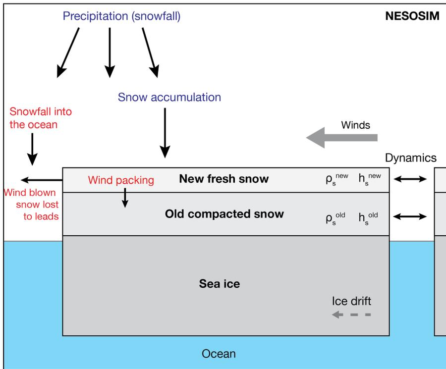
**Figure 1:** Schematic of the NASA Eulerian Snow On Sea Ice Model (NESOSIM) presented in this study. The red (blue) text indicates processes that result in a loss (gain) of snow. 'Dynamics' indicates the combination of ice/snow advection and convergence/divergence which can cause either loss or gain of snow.
