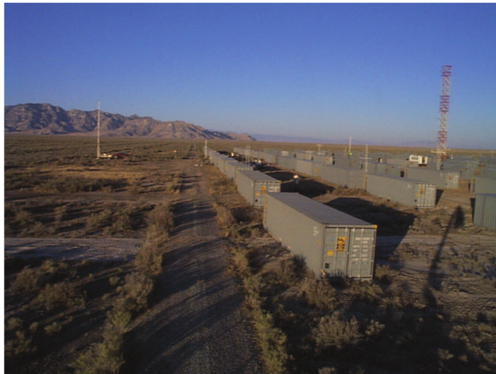
Figure 20. (a) Photograph of the MUST containers in the Utah's West desert; (b) Schematic representation of the containers layout. The location of the concentration (detectors) and wind sensors (S and T towers) are indicated, as well as the position (red cross) of the pollutant release and the direction of the incoming flow (green arrow) of the case 2681829. Source: Biltoft (2001) and Yee and Biltoft (2004).
