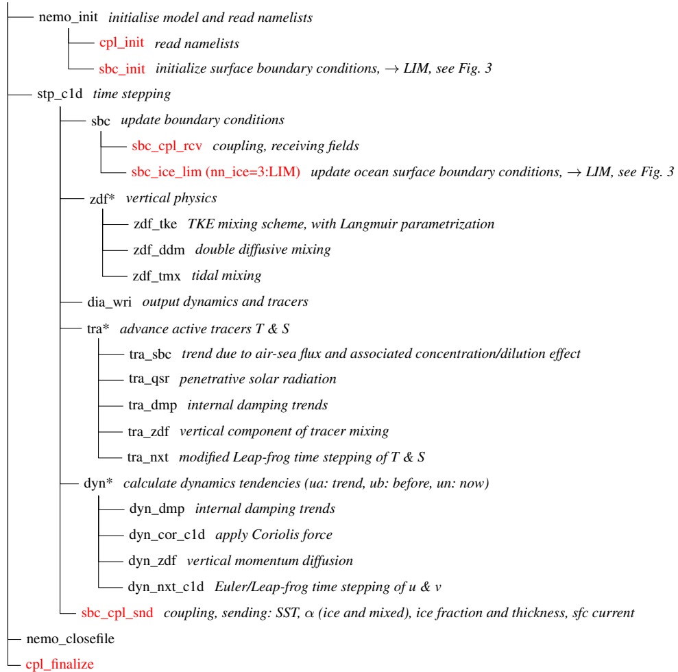
Figure 2. Simplified flow chart of the NEMO model. Routines dedicated to coupling via OASIS are coloured red.
