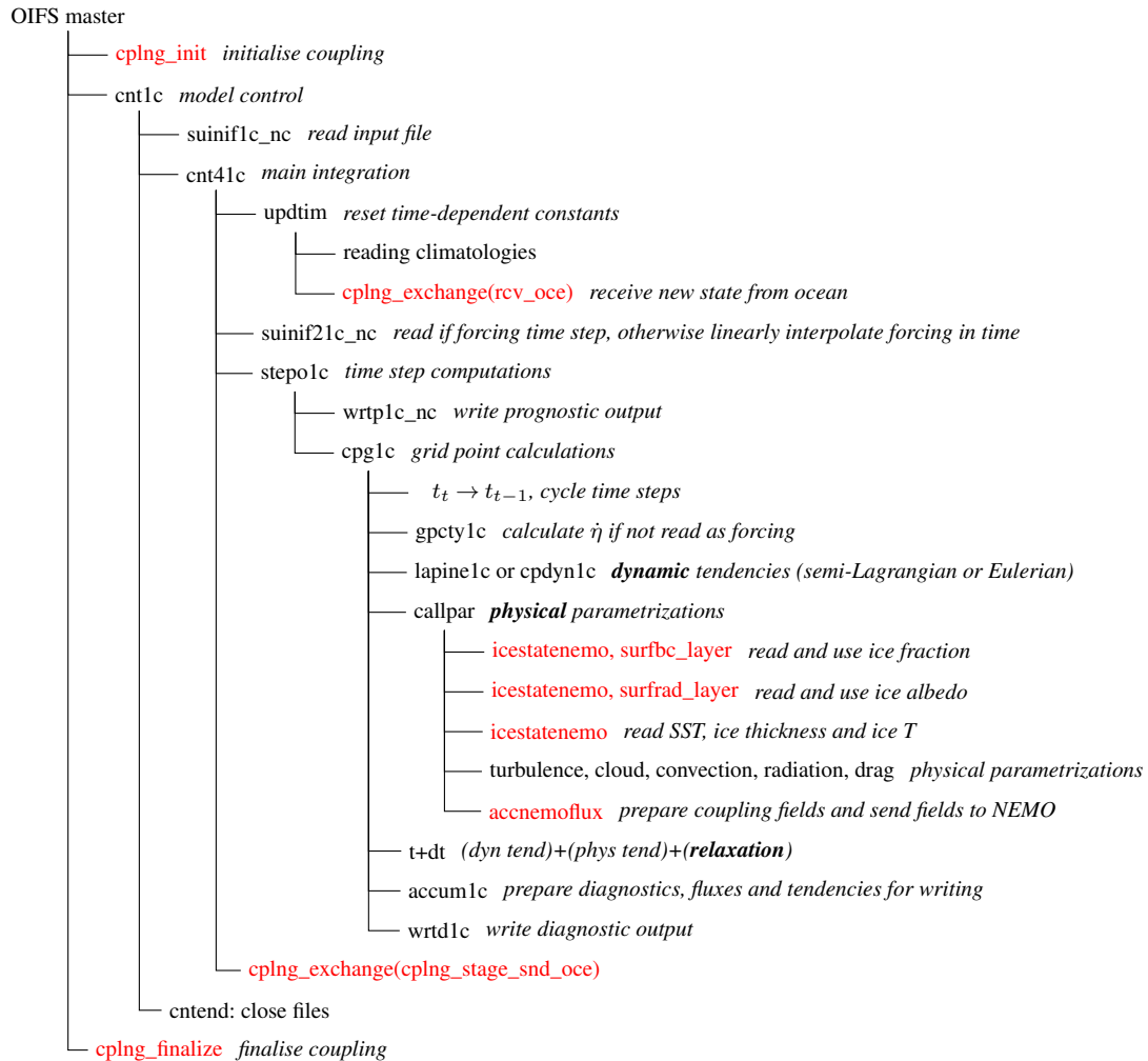
Figure 1. Simplified flow chart of the OIFS model. Routines dedicated to coupling via OASIS are coloured red.
