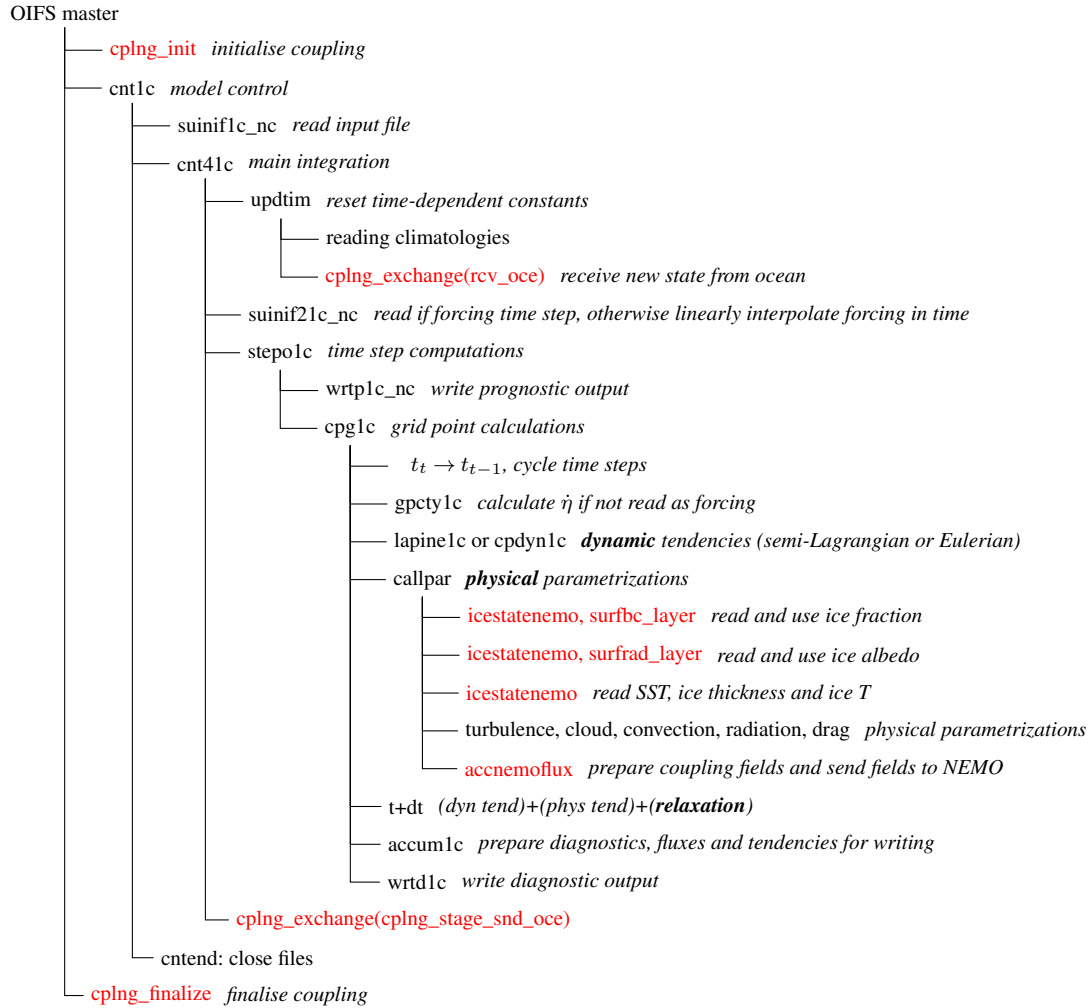
Figure 1. Flow-Simplified flow chart of the OIFS model. Routines dedicated to coupling via OASIS are coloured red.
