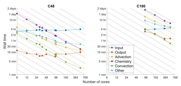
15 Figure 4. Total wall time per component for a low (C48) and high (C180) resolution simulation. Simulations at C180 are limited to core counts of 90 or more across several nodes for the hardware used here, due to the high memory requirements of such high-resolution simulations.
